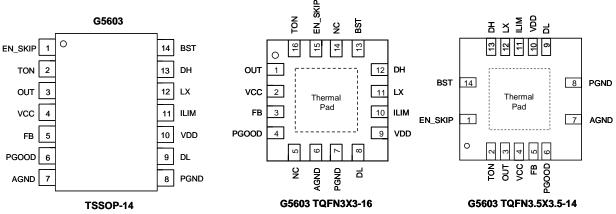
Note: Recommend connecting the Thermal Pad to the Ground for excellent power dissipation.
