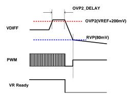
Figure 15: OVP and RVP Fault Protection
