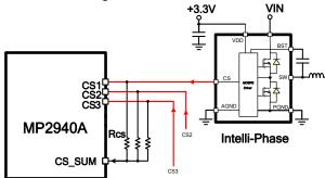
Figure 7: Phase Current Sense with 3-phase Configuration
