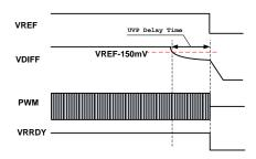
Figure 18: Under-Voltage Protection
