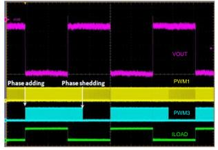
Figure 12: Phase Shedding and Adding Process
