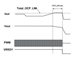
Figure 16: OC Protection for Total Current
