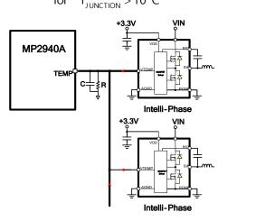
Figure 10: External Temperature Sense
