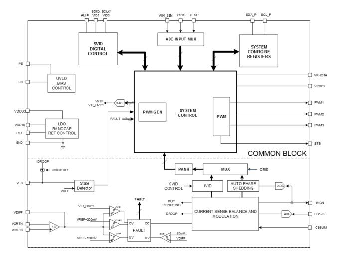
Figure 3: System Functional Block
