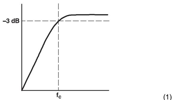
The value of  $C_i$  is important to consider as it directly affects the low-frequency, or bass, performance of the circuit. Furthermore, the input impedance changes with a change in volume. The higher the volume, the lower the input impedance is. To determine the appropriate capacitor value, reconfigure Equation 1 into Equation 2. The value of the input resistor,  $R_i$ , can be determined from Equation 2.
