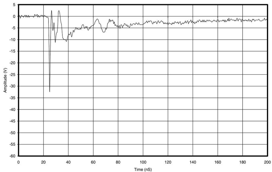
**Figure 5. IEC Clamping Waveforms
