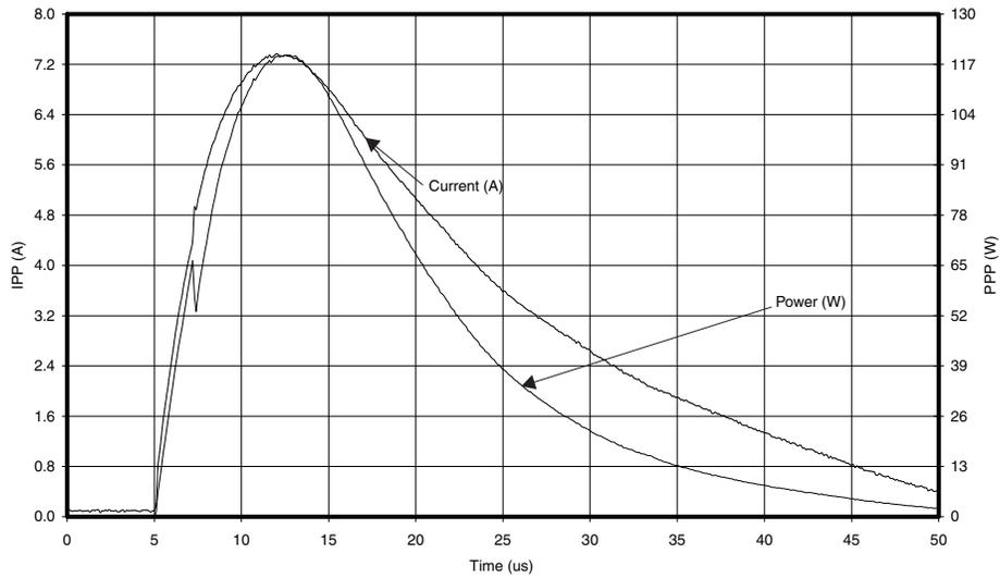
Figure 2. Peak Pulse Waveforms
