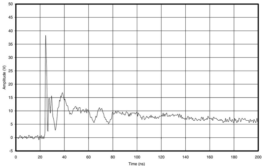
**Figure 4. IEC Clamping Waveforms
