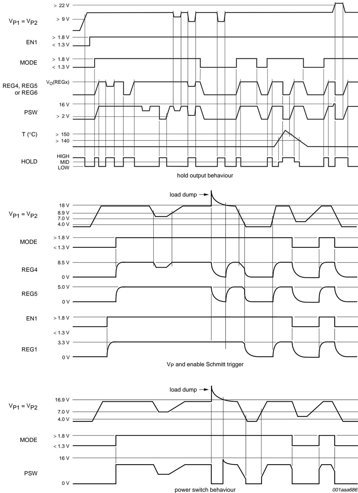
Fig 5. Timing diagram of the HOLD output, V<sub>P</sub> and Schmitt trigger and power switch
