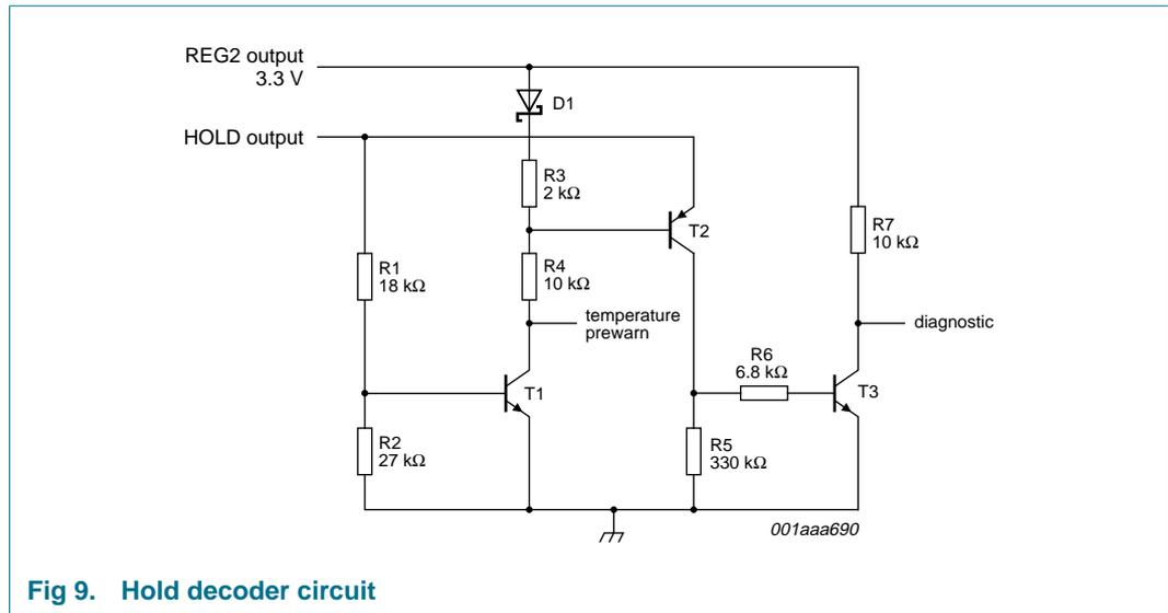
Fig 9. Hold decoder circuit
