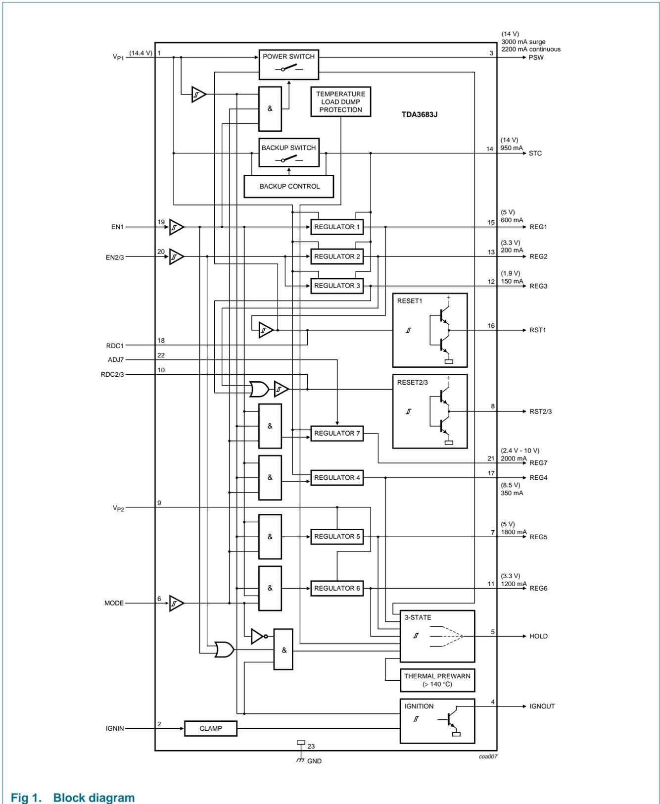
Fig 1. Block diagram
