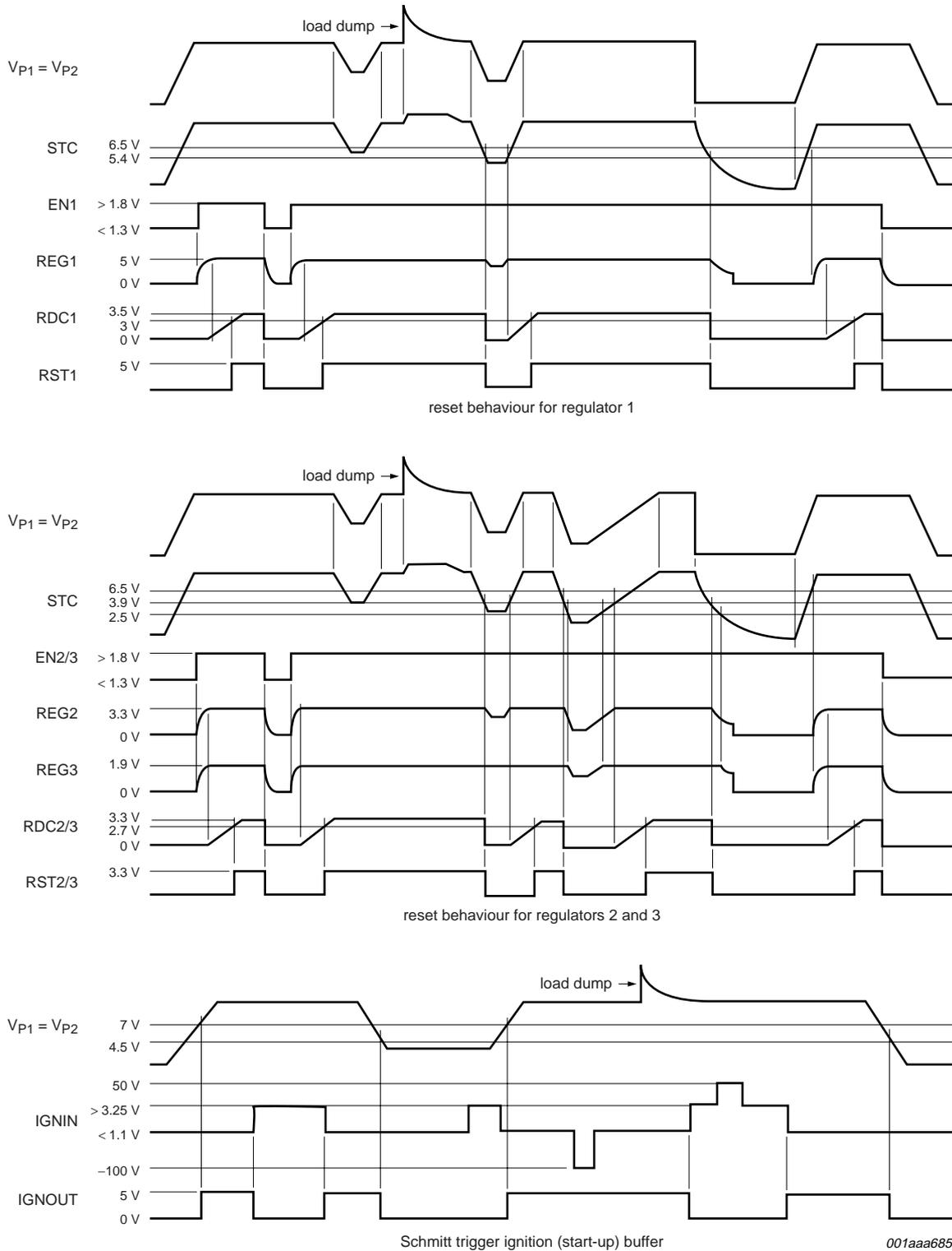
Fig 4. Timing diagram of the reset outputs for REG1, REG2 and REG3 and ignition Schmitt trigger
