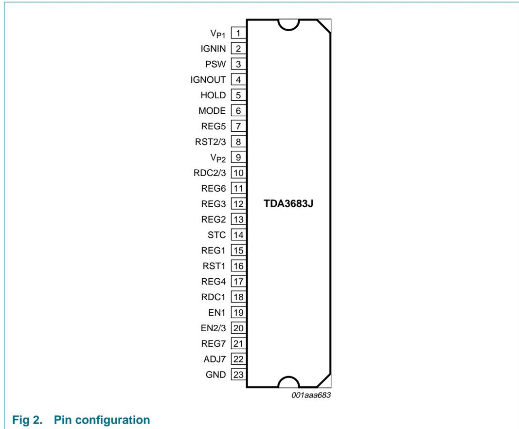
Fig 2. Pin configuration
