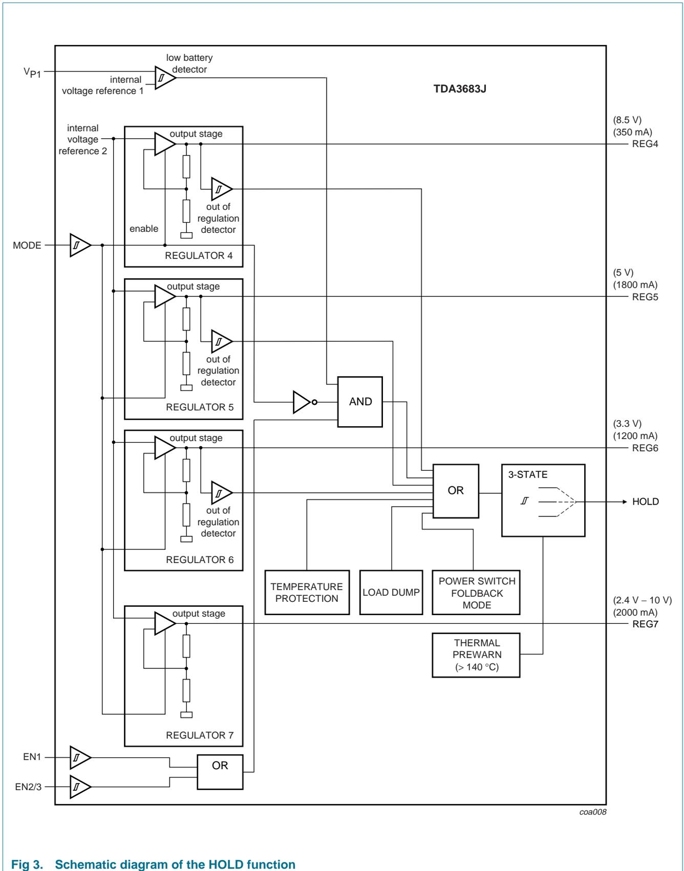
Fig 3. Schematic diagram of the HOLD function
