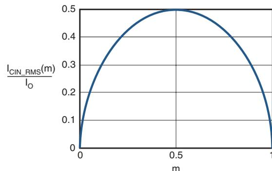
Figure 2.  $I_{CIN}$  vs. Voltage Conversion Ratio
