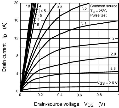
**Fig. 8.1  $I_D - V_{DS}$**
