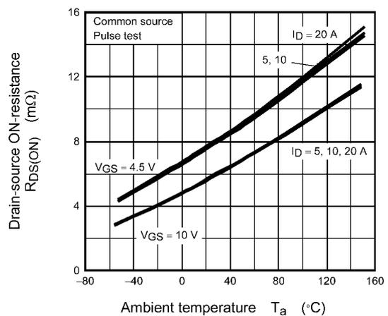
**Fig. 8.6  $R_{DS(ON)} - T_a$**
