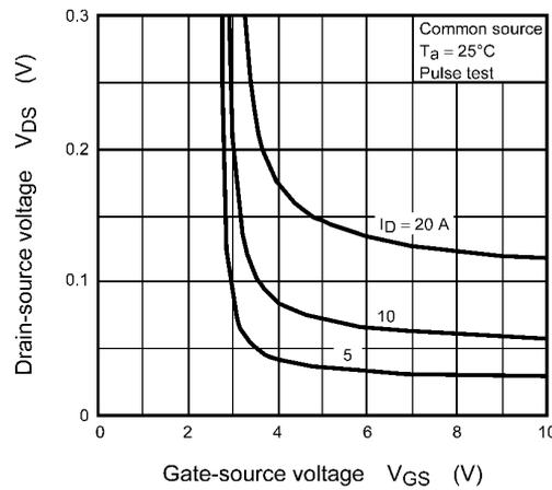
**Fig. 8.4  $V_{DS} - V_{GS}$**
