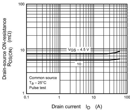
**Fig. 8.5  $R_{DS(ON)} - I_D$**
