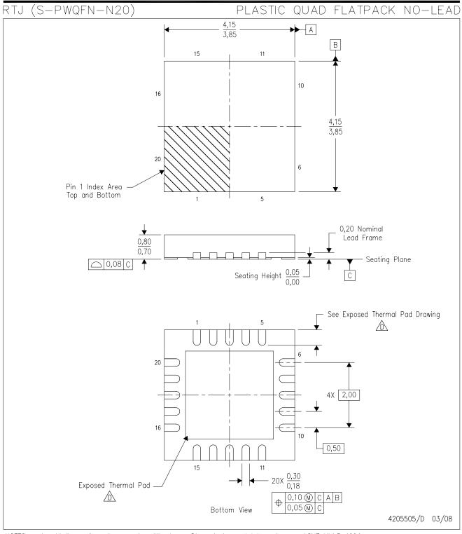
NOTES: A. All linear dimensions are in millimeters. Dimensioning and tolerancing per ASME Y14.5-1994.
