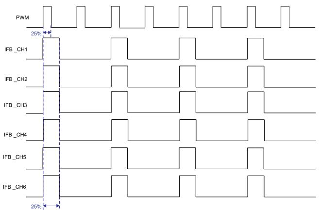
Figure 18. Programmable PWM Dimming Timing Diagram
