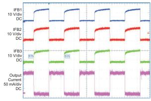
Figure 11. Programmable PWM Waveform
