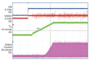
Figure 15. Start Up Waveform
