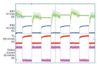
Figure 12. Output Ripple Waveform
