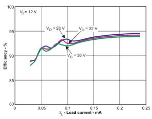
Figure 1. Efficiency vs Load Current by Output Voltage
