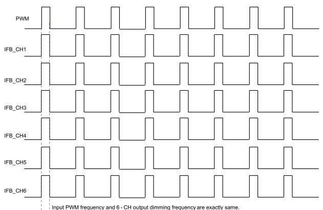
Figure 19. Direct PWM Dimming Timing Diagram
