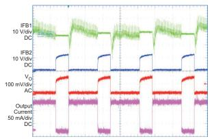
Figure 13. Output Ripple Waveform
