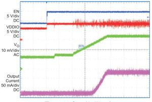
Figure 14. Start Up Waveform
