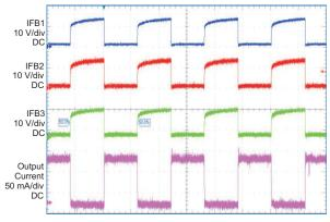
Figure 10. Programmable PWM Waveform
