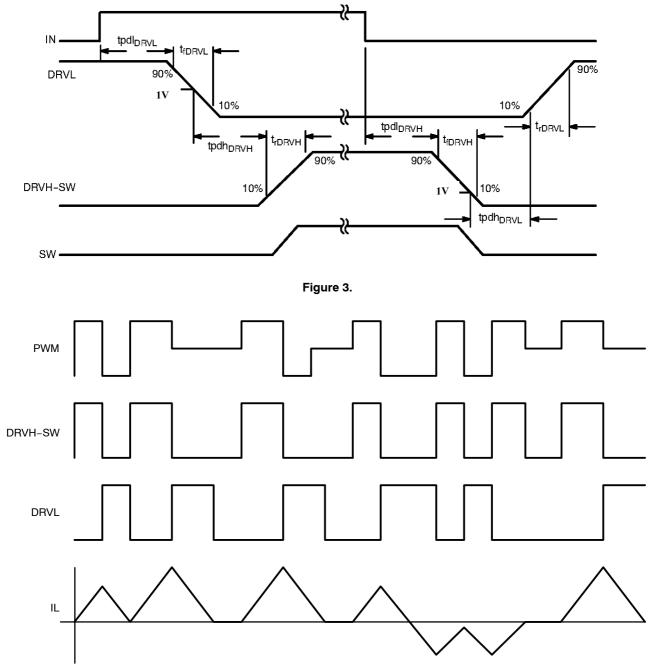
Figure 4. Timing Diagram
