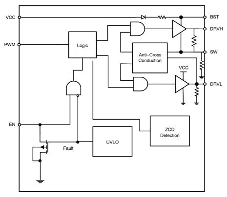
Figure 1. Block Diagram
