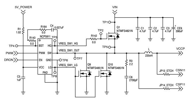
Figure 2. Application Circuit
