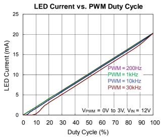
Figure 7. LED Current vs. PWM Dimming Duty Cycle
