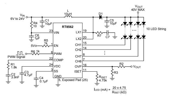
Figure 1. 1MHz, 20mA Full Scale Current PWM Dimming Control
