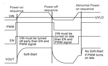
Figure 5. Power-On Sequence Control by VIN
