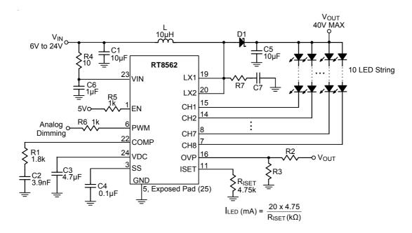
Figure 2. 1MHz, 20mA Full Scale Current Analog Dimming Control
