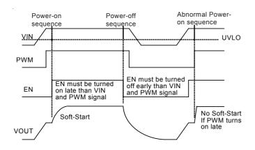
Figure 4. Power-On Sequence Control by EN
