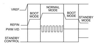
Figure 9. PWM VID Time Diagram
