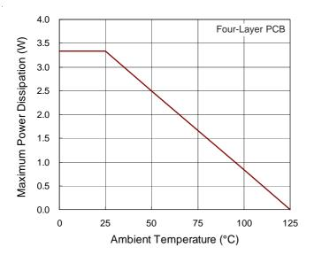
Figure 12. Derating Curve of Maximum Power Dissipation
