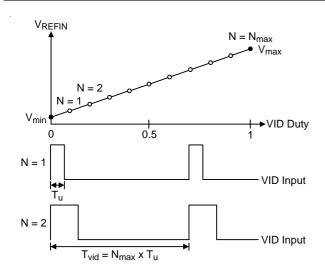
Figure 10. PWM VID Analog Output
