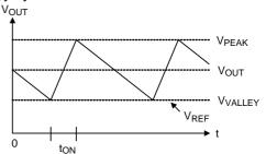
Figure 4. Constant On-Time PWM Control
