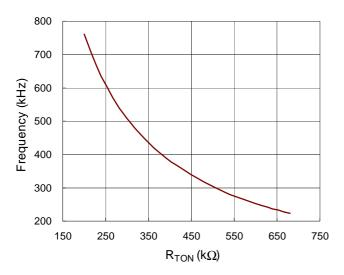
Figure 5. Frequency vs. R<sub>TON</sub>
