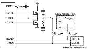
Figure 3. Output Voltage Sensing
