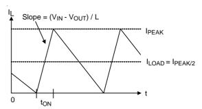
Figure 6. Boundary condition of CCM/DEM
