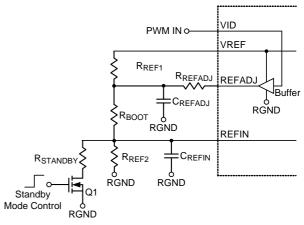
Figure 8. PWM VID Analog Circuit Diagram
