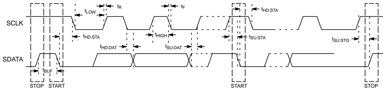
Figure 3. I<sup>2</sup>C Timing Diagram
