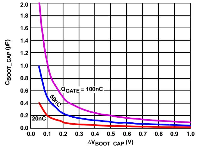
FIGURE 8. BOOTSTRAP CAPACITANCE vs BOOT RIPPLE VOLTAGE
