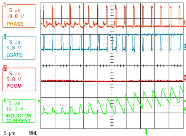
FIGURE 2. LOAD TRANSIENT (0 - 30A, 3-PHASE)
