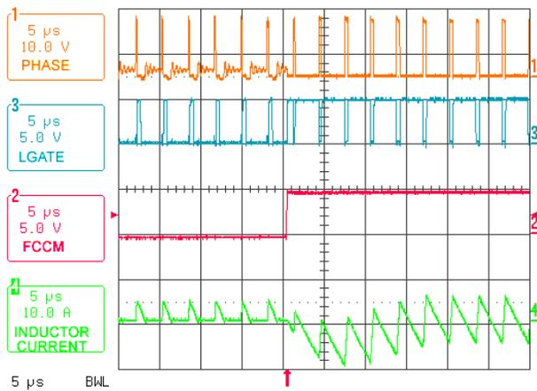
FIGURE 4. DCM TO CCM TRANSITION AT NO LOAD
