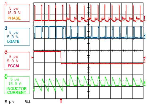
FIGURE 5. CCM TO DCM TRANSITION AT NO LOAD
