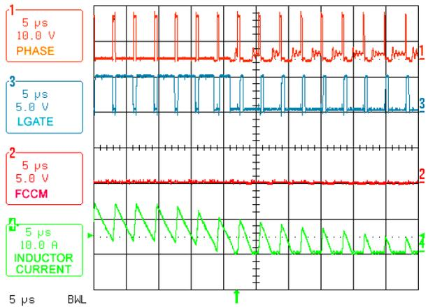
FIGURE 3. LOAD TRANSIENT (30 - 0A, 3-PHASE)
