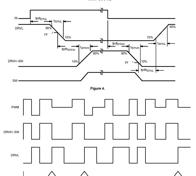
Figure 5. Timing Diagram
