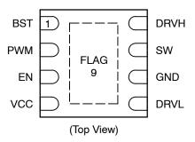
Figure 1. Pin Diagram
