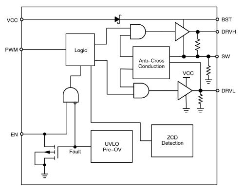
Figure 2. Block Diagram
