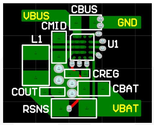
Figure 51. PCB Layout Recommendations
