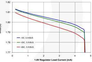
Figure 20. V<sub>REG</sub> 1.8V Output Regulation
