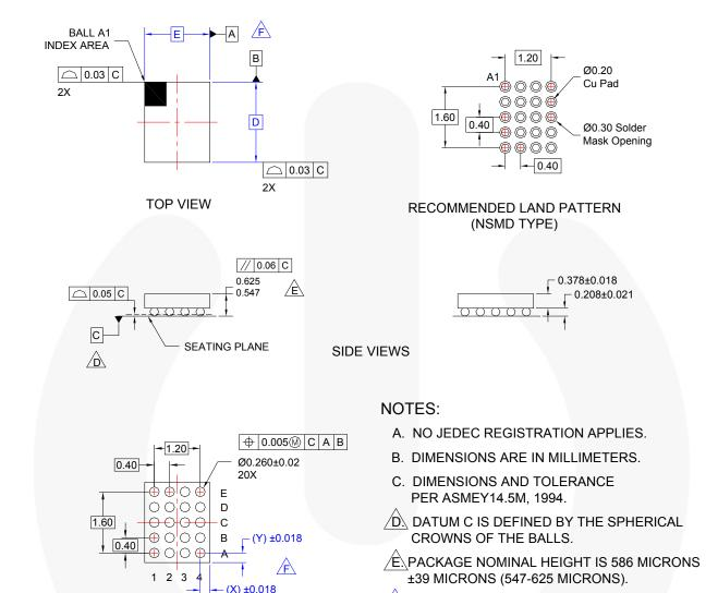
Figure 52. 20-Ball WLCSP, 4X5 Array, 0.4mm Pitch, 250µm Ball
