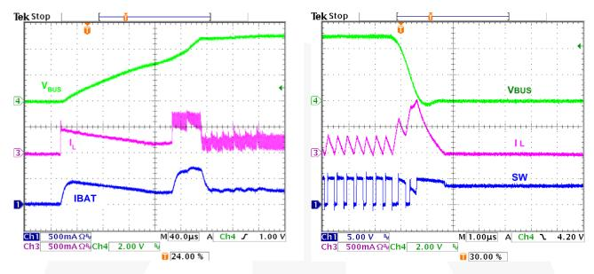
Figure 31. Startup, 3.6V<sub>BAT</sub>, 44 $\Omega$  Load, Additional 10 $\mu$ F, X5R Across V<sub>BUS</sub>
