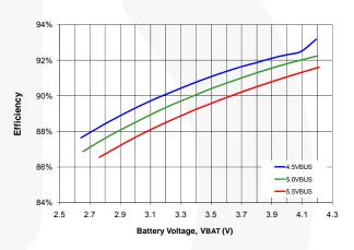
Figure 9. Charger Efficiency, No I<sub>INLIM</sub>, I<sub>OCHARGE</sub>=1,450mA
