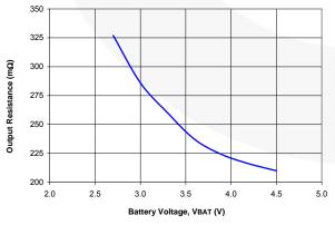
Figure 43. Output Resistance (ROUT)
