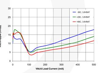
Figure 30. Output Ripple vs. Temperature
