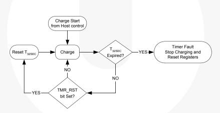
Figure 42. Timer Flow Chart for FAN54011 and FAN54014
