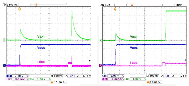
Figure 17. No Battery at V<sub>BUS</sub> Power-up; FAN54010, FAN54013
