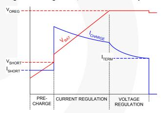
Figure 36. Charge Curve, IINLIM Limits ICHARGE
