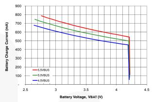
Figure 7. Battery Charge Current vs.  $V_{\text{BUS}}$  with  $I_{\text{INLIM}} = 100 \text{mA}$
