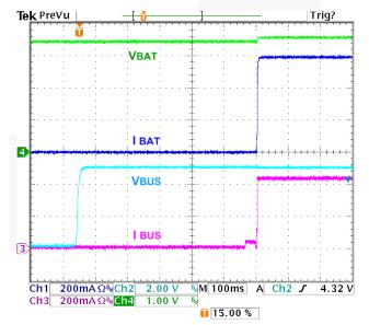
Figure 11. Auto-Charge Startup at  $V_{\text{BUS}}$  Plug-in,  $I_{\text{INLIM}} \! = \! 100 \text{mA}, \, \text{OTG=1}, \, V_{\text{BAT}} \! = \! 3.4 \text{V}$
