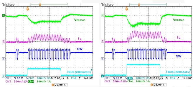
Figure 33. Load Transient, 5-155-5mA, t<sub>R</sub>=t<sub>F</sub>=100ns
