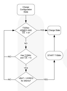
Figure 39. Charge Configuration
