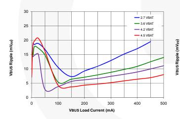
Figure 29. Output Ripple vs. V<sub>BAT</sub>
