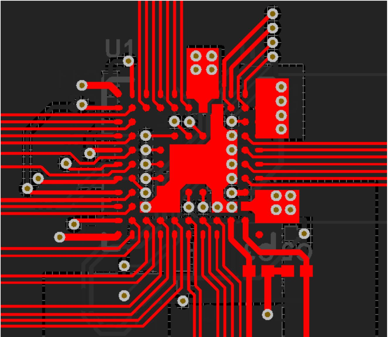
Figure 103. Final Routing and GND Pour (Top Layer)
