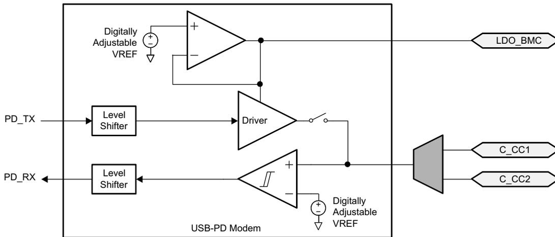
Figure 14. USB-PD BMC TX/Rx Block Diagram
