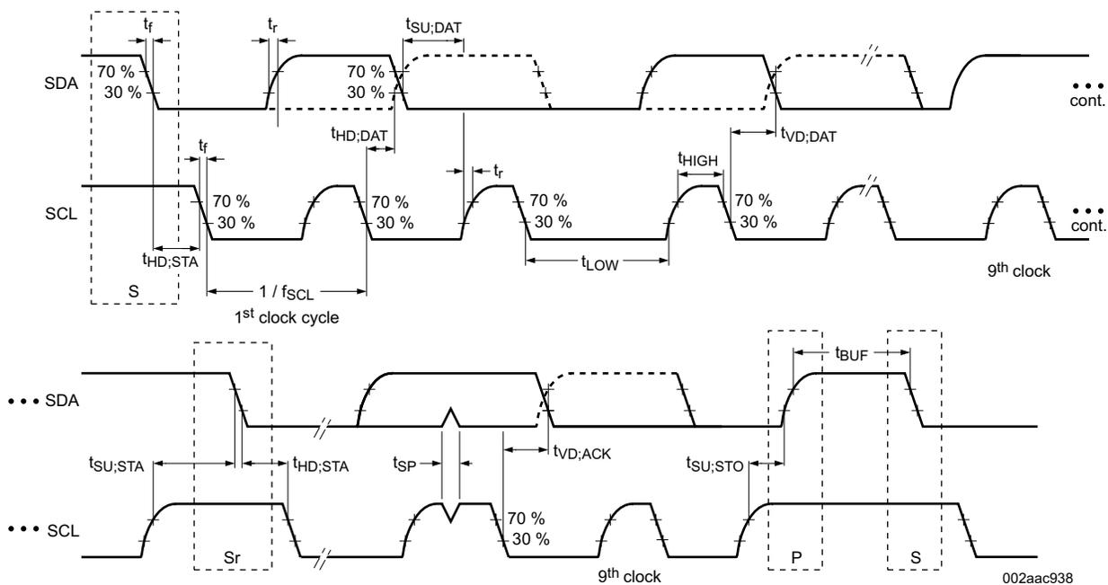
Figure 7. I<sup>2</sup>C Slave Interface Timing
