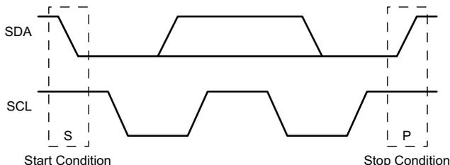
Figure 70. I<sup>2</sup>C Definition of Start and Stop Conditions
