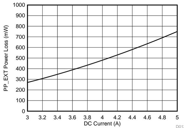
**Figure 78. PP\_EXT Power Loss ( $R_{NFETS} + R_{SENSE} = 30\text{ m}\Omega$ )**
