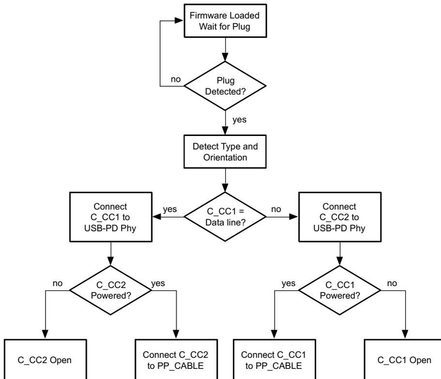
Figure 37. Port C\_CC and VCONN Connection Flow
