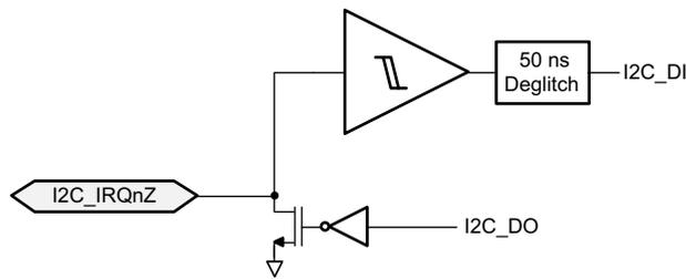
Figure 60. IOBUF\_I2C I/O
