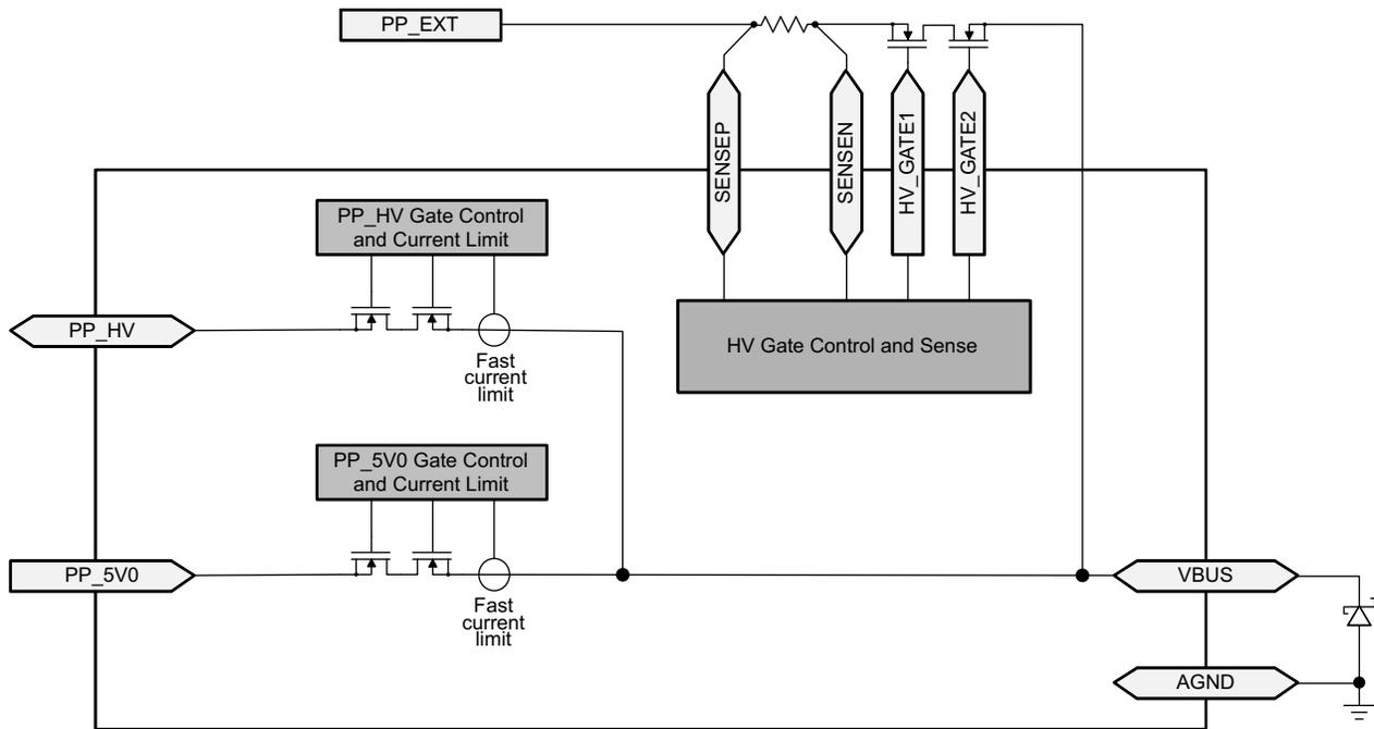
Figure 86. Schottky on VBUS for Current Surge Protection
