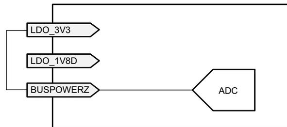
**Figure 31. BUSPOWERZ Configured to Disable Power from VBUS**
