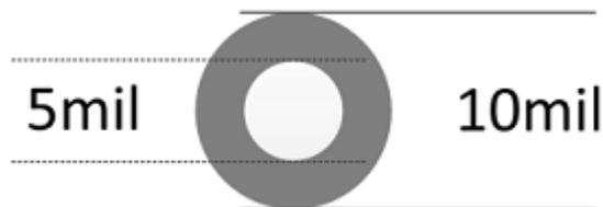
Figure 88. Under Ball Recommended Via Size
