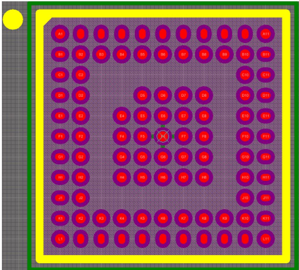
Figure 89. Top View Alternate TPS65982 Footprint (Oval Pads)
