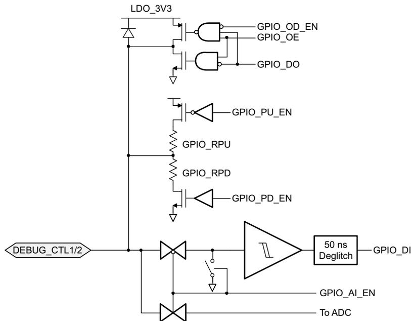
Figure 55. IOBUF\_GPIOLS<sub>I2C</sub> (General GPIO) I/O with I<sup>2</sup>C De-glitch
