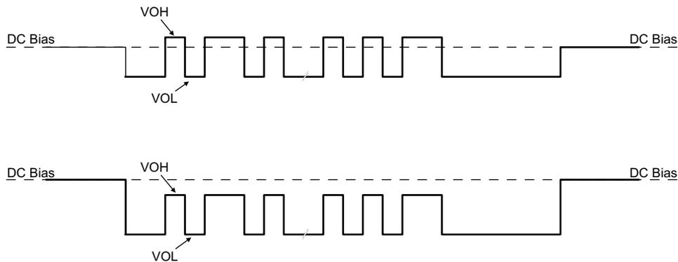
Figure 15. TX Driver Transmission with DC Bias
