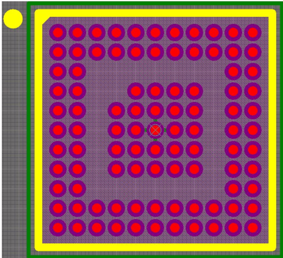
Figure 87. Top View Standard TPS65982 Footprint (Circular Pads)
