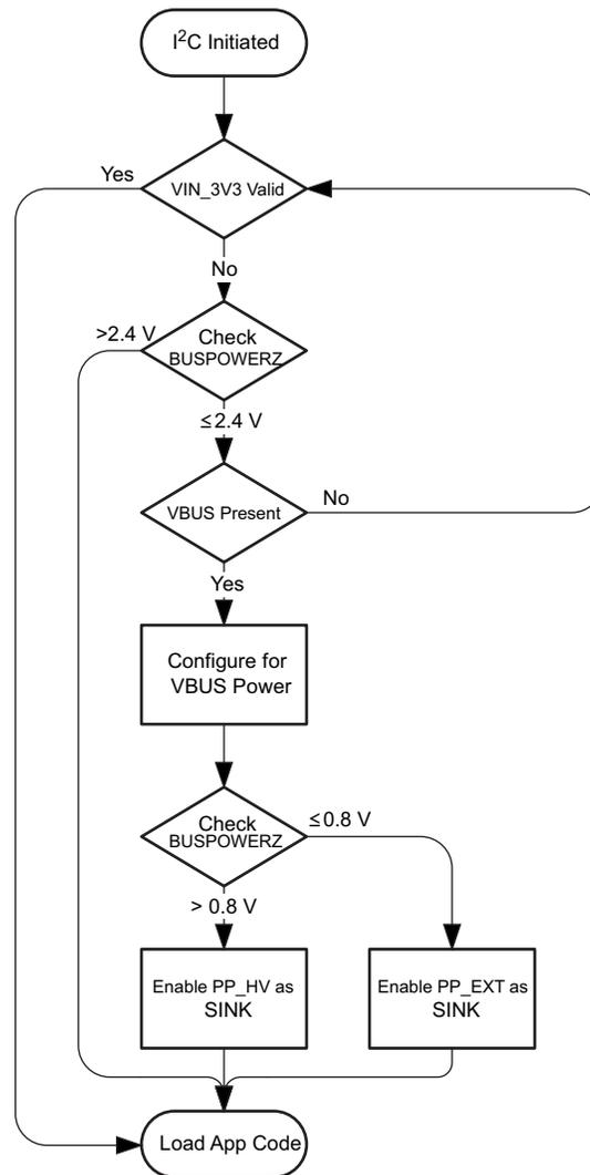
**Figure 65. Dead-Battery Condition Flow Diagram**
