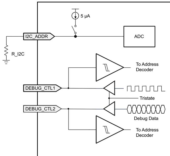
Figure 76. I<sup>2</sup>C Address Decode
