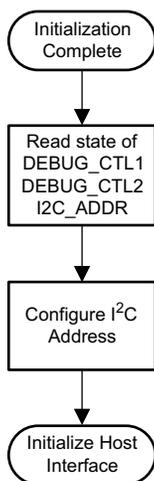
Figure 64. I<sup>2</sup>C Address Configuration
