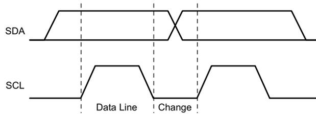
**Figure 71. I<sup>2</sup>C Bit Transfer**
