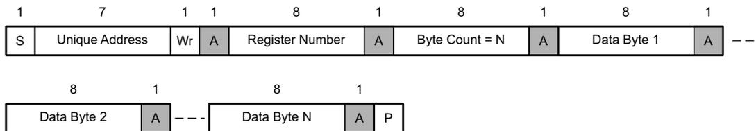
Figure 73. I<sup>2</sup>C Unique Address Write Register Protocol
