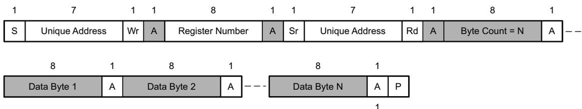
Figure 74. I<sup>2</sup>C Unique Address Read Register Protocol
