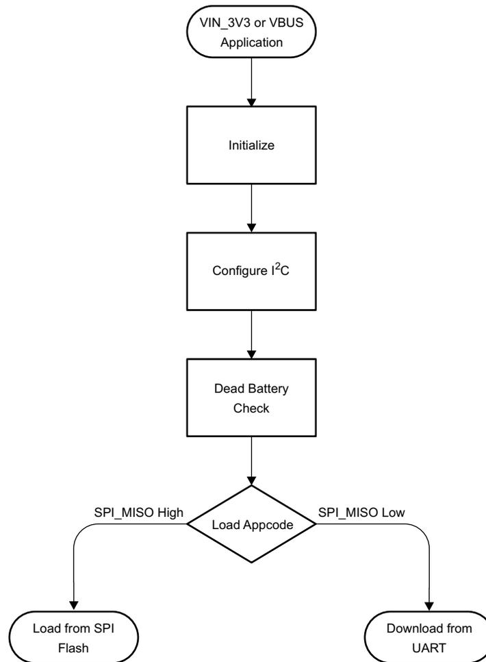
**Figure 63. Flow Diagram for Boot Code Sequence**
