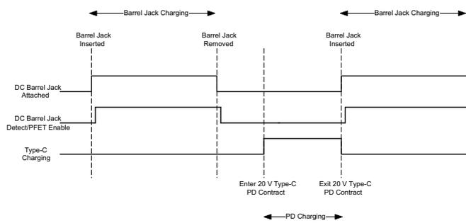
Figure 83. DC Barrel Jack and Type-C PD Charging Hand-Off
