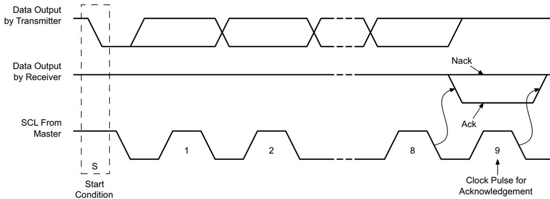
**Figure 72. I<sup>2</sup>C Acknowledgment**
