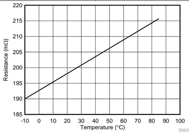
Figure 3. PP\_CABLE Switch On-Resistance vs. Temperature
