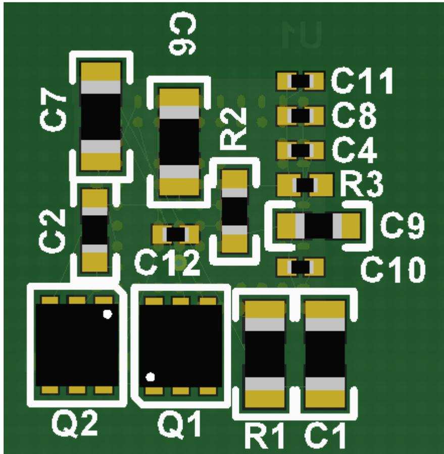
Figure 95. Example Layout (Bottom View in 3-D)
