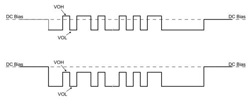
Figure 15. TX Driver Transmission with DC Bias
