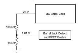
Figure 80. DC Barrel Jack Voltage Divider
