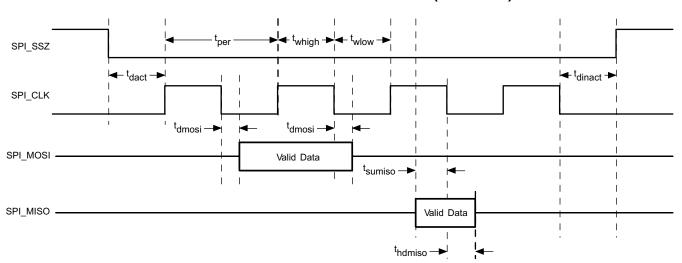
Figure 8. SPI Master Timing
