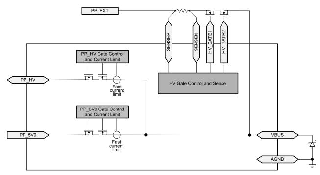
Figure 86. Schottky on VBUS for Current Surge Protection
