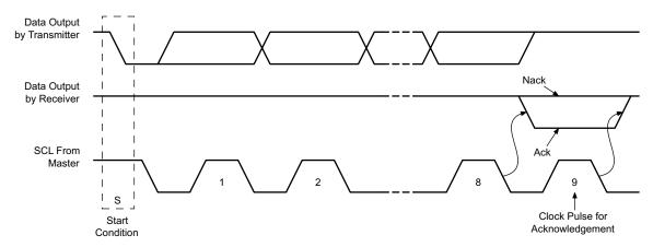
Figure 72. I<sup>2</sup>C Acknowledgment
