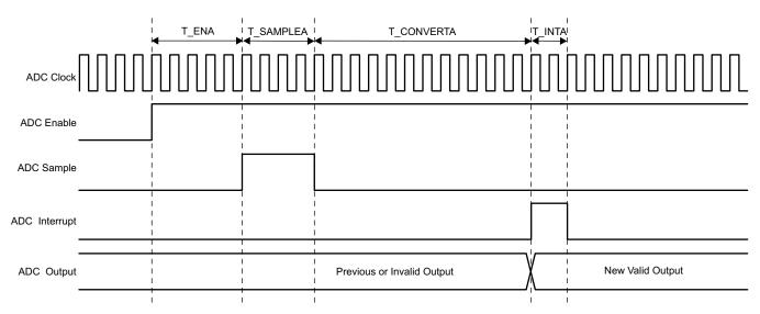
Figure 5. ADC Enable and Conversion Timing
