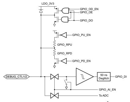
Figure 55. IOBUF\_GPIOLSI2C (General GPIO) I/O with I<sup>2</sup>C De-glitch
