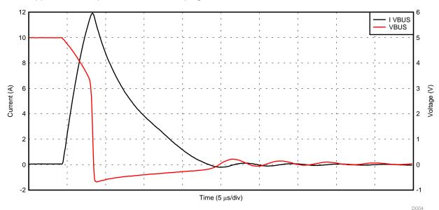
Figure 22. PP\_5V0 Current Limit with a Hard Short
