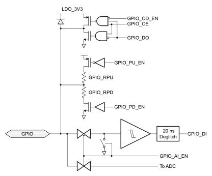
Figure 54. IOBUF\_GPIOLS (General GPIO) I/O
