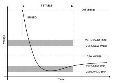
Figure 35. Negative Voltage Transition on VBUS
