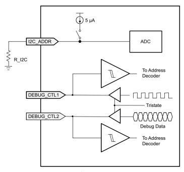
Figure 76. I<sup>2</sup>C Address Decode
