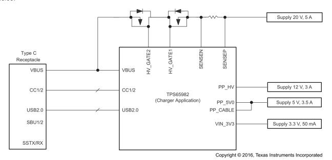
Figure 77. Type-C and PD Charger Application
