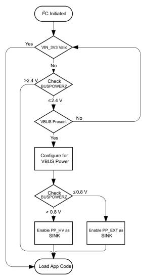
Figure 65. Dead-Battery Condition Flow Diagram
