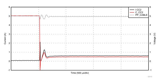
Figure 41. PP\_CABLE to C\_CCn Current Limit with a Hard Short (Extended Time Base)
