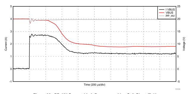
Figure 28. PP\_HV Current Limit Response with a Soft Short (7  $\Omega$ )
