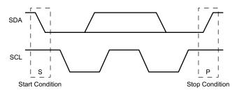
Figure 70. I<sup>2</sup>C Definition of Start and Stop Conditions
