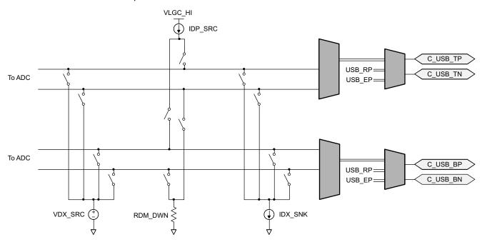
Figure 48. BC1.2 Detection Circuitry
