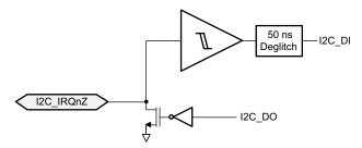
Figure 60. IOBUF\_I2C I/O
