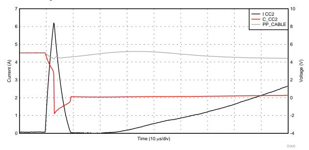
Figure 40. PP\_CABLE to C\_CCn Current Limit with a Hard Short
