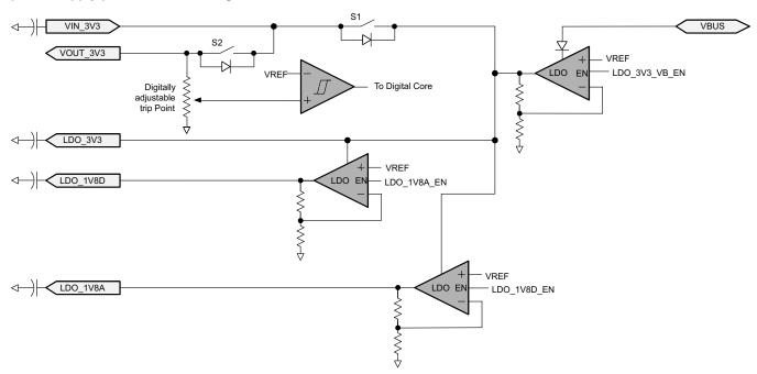
Figure 49. Power Supply Path
