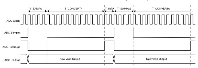
Figure 6. ADC Repeated Conversion Timing
