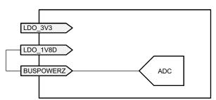
Figure 32. BUSPOWERZ Configured with PP\_HV as Input Power Path
