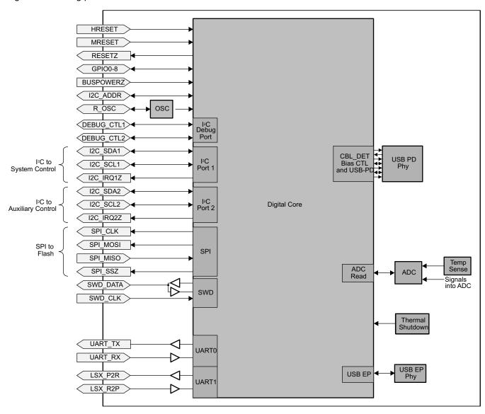
Figure 50. Digital Core Block Diagram
