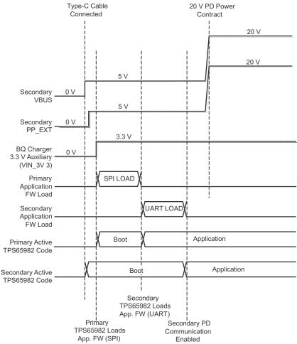
Figure 85. Secondary TPS65982 Dead Battery Sequence
