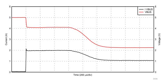
Figure 24. PP\_5V0 Current Limit with a Soft Short (2  $\Omega$ )
