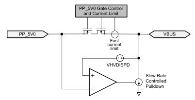
Figure 36. PP 5V0 Slew Rate Control
