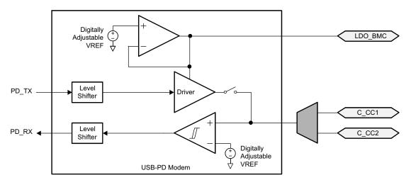
Figure 14. USB-PD BMC TX/Rx Block Diagram
