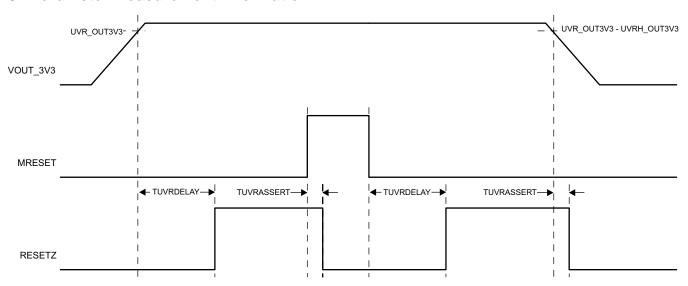
Figure 4. RESETZ Assertion Timing
