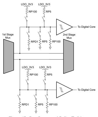
Figure 45. Port Detect and Pullup/Pulldown
