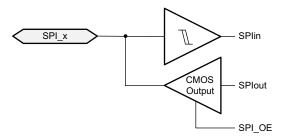
Figure 61. IOBUF\_GPIOHSSPI
