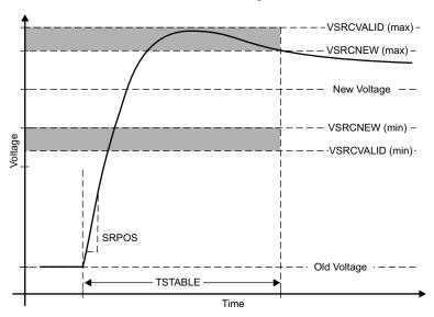
Figure 34. Positive Voltage Transition on VBUS
