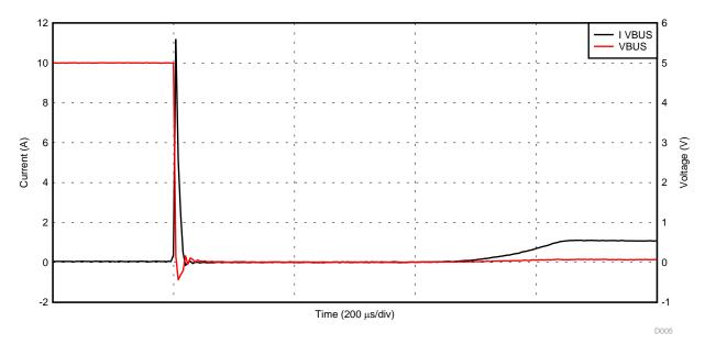
Figure 23. PP\_5V0 Current Limit with a Hard Short (Extended Time Base)
