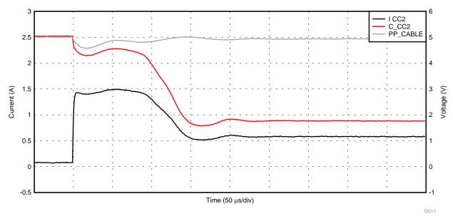
Figure 42. PP\_CABLE to C\_CCn Current Limit Response with a Soft Short (2  $\Omega$ )
