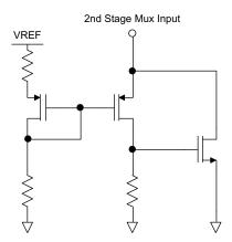
Figure 46. Port Mux Clamp
