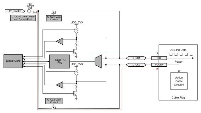
Figure 38. Port C\_CC1 and C\_CC2 Normal Orientation Power from PP\_CABLE
