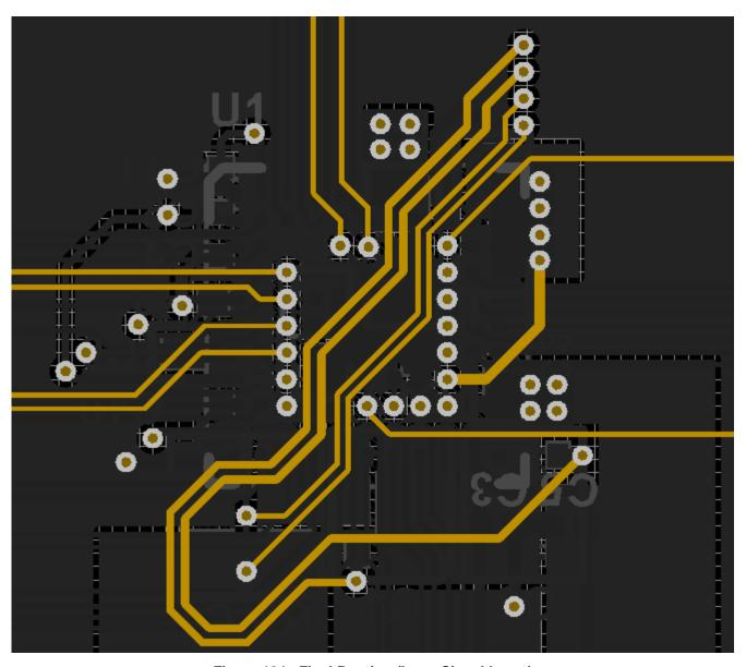
Figure 104. Final Routing (Inner Signal Layer)
