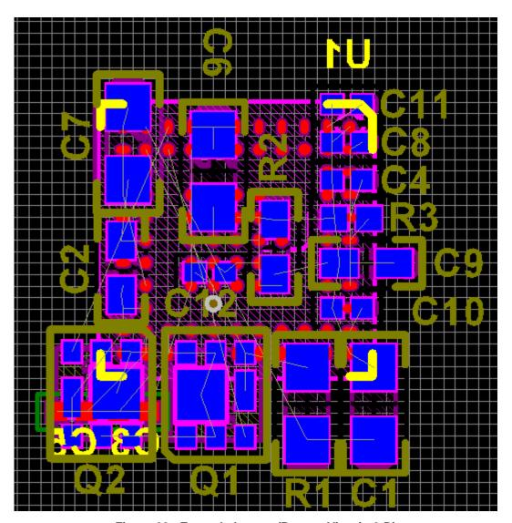
Figure 93. Example Layout (Bottom View in 2-D)
