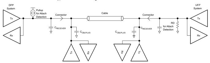
Figure 17. Example USB-PD Multi-Drop Configuration
