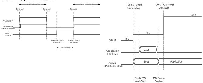
Figure 83. DC Barrel Jack and Type-C PD Charging Hand-Off
