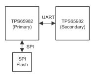
Figure 82. Primary and Secondary TPS65982 Sharing a Single Flash
