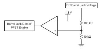
Figure 81. Barrel Jack Detect Comparator
