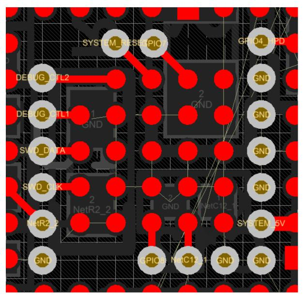
Figure 101. Void Via Placement
