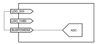
Figure 31. BUSPOWERZ Configured to Disable Power from VBUS
