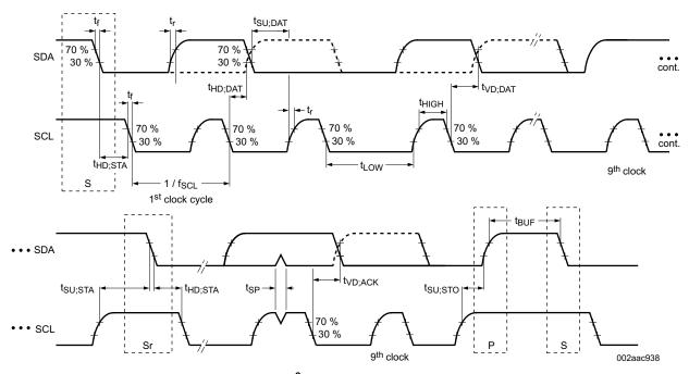
Figure 7. I<sup>2</sup>C Slave Interface Timing
