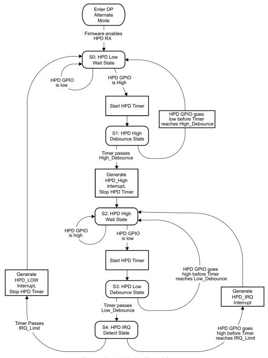
Figure 52. HPD TX Flow Diagram
