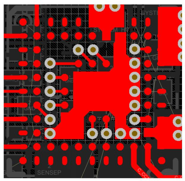
Figure 102. Top Layer GND Pour
