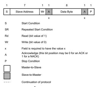
Figure 75. I<sup>2</sup>C Read/Write Protocol Key
