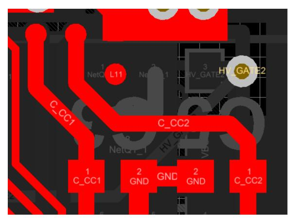
Figure 98. CC1 and CC2 Capacitor Routing
