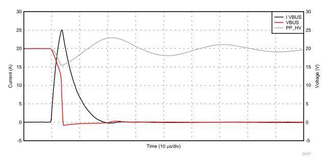
Figure 27. PP\_HV Current Limit Response with a Hard Short
