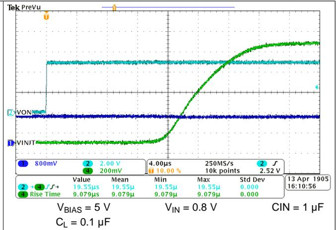
Figure 28.  $t_R$  at  $V_{BIAS} = 5\text{ V}$
