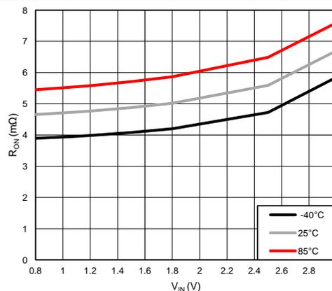
$V_{BIAS} = 5\text{ V}$        $V_{ON} = 5\text{ V}$        $I_{OUT} = -6\text{ A}$
