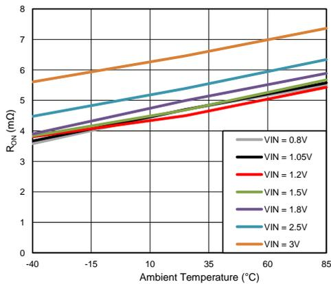
$V_{BIAS} = 5\text{ V}$        $V_{ON} = 5\text{ V}$        $I_{OUT} = -200\text{ mA}$
