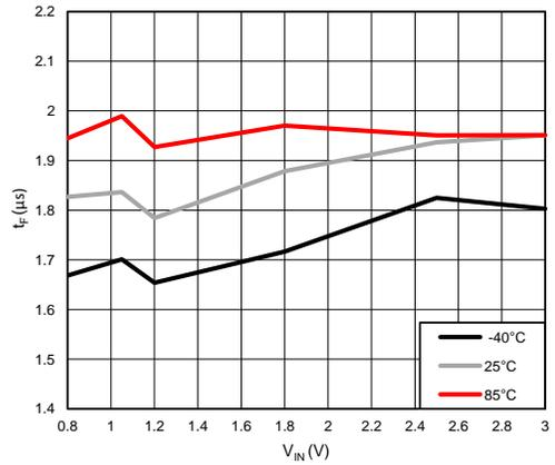
$V_{BIAS} = 5V$        $R_L = 10\Omega$        $C_L = 0.1\mu F$
