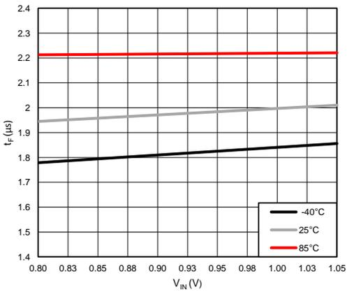
$V_{BIAS} = 3V$        $R_L = 10\Omega$        $C_L = 0.1\mu F$
