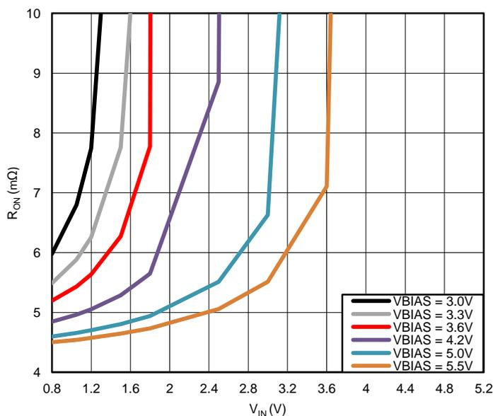
Figure 25.  $R_{ON}$  vs  $V_{IN}$  ( $V_{IN} > V_{BIAS}$ )
