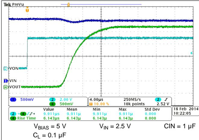
Figure 27.  $t_R$  at  $V_{BIAS} = 5\text{ V}$
