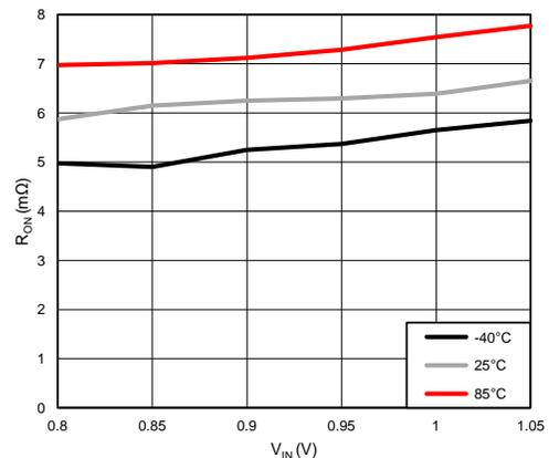
$V_{BIAS} = 3\text{ V}$        $V_{ON} = 5\text{ V}$        $I_{OUT} = -200\text{ mA}$
