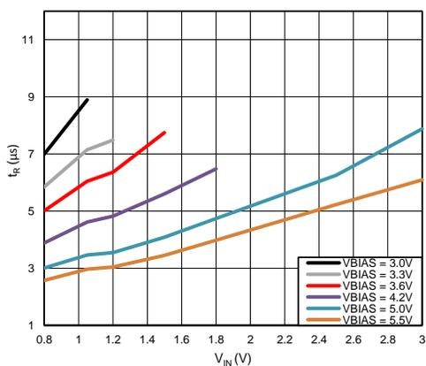
T<sub>A</sub> = 25°C      R<sub>L</sub> = 10 Ω      C<sub>L</sub> = 0.1 μF
