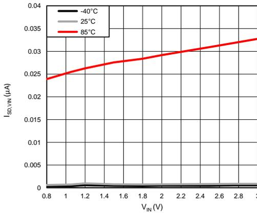
$V_{BIAS} = 5\text{ V}$        $V_{ON} = 0\text{ V}$        $V_{OUT} = 0\text{ V}$
