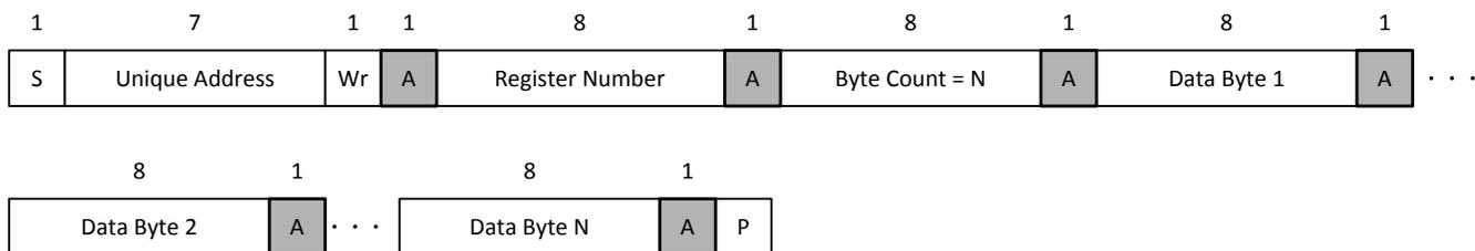
**Figure 29. I<sup>2</sup>C Unique Address Write Register Protocol**
