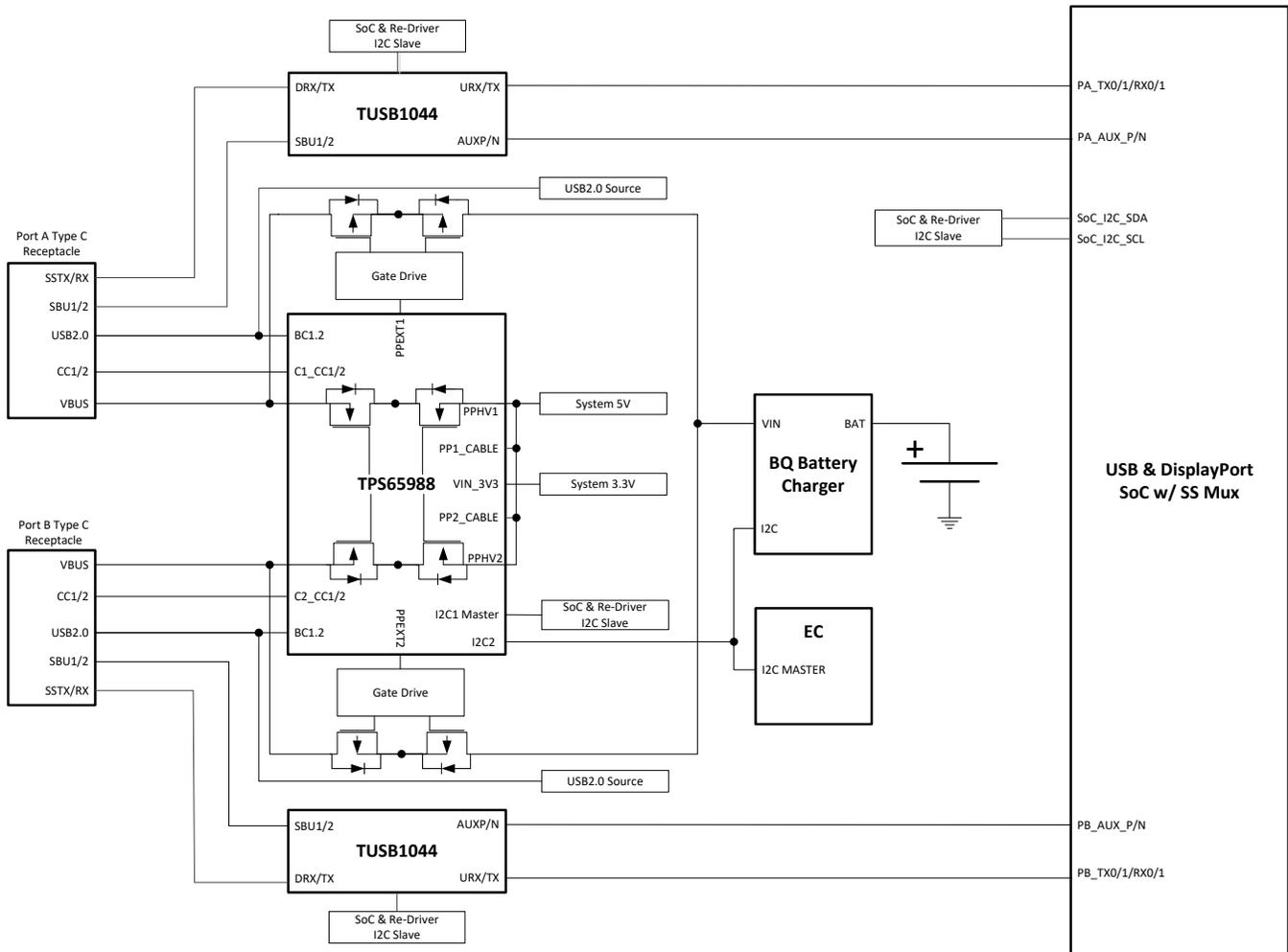
Figure 42. TPS65988 and SoC & Redriver I2C
