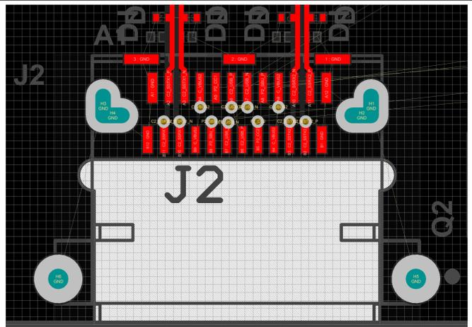
Figure 50. Type-C Connector SSTXR Top Layer
