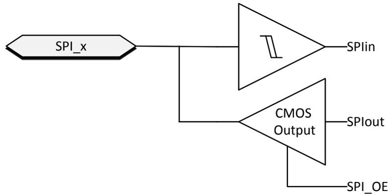
**Figure 24. SPI buffer**
