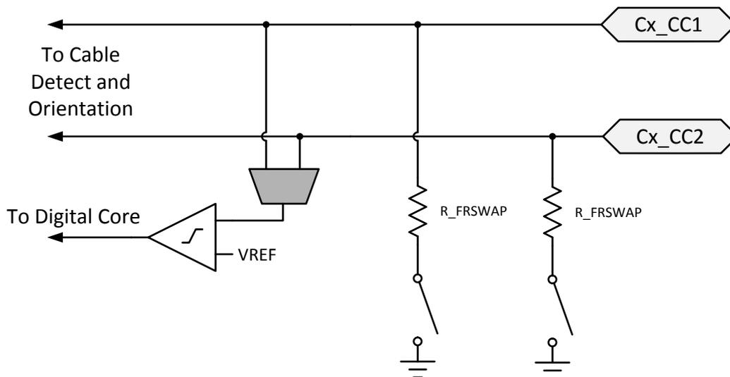
Figure 18. Fast Role Swap Detection and Signaling
