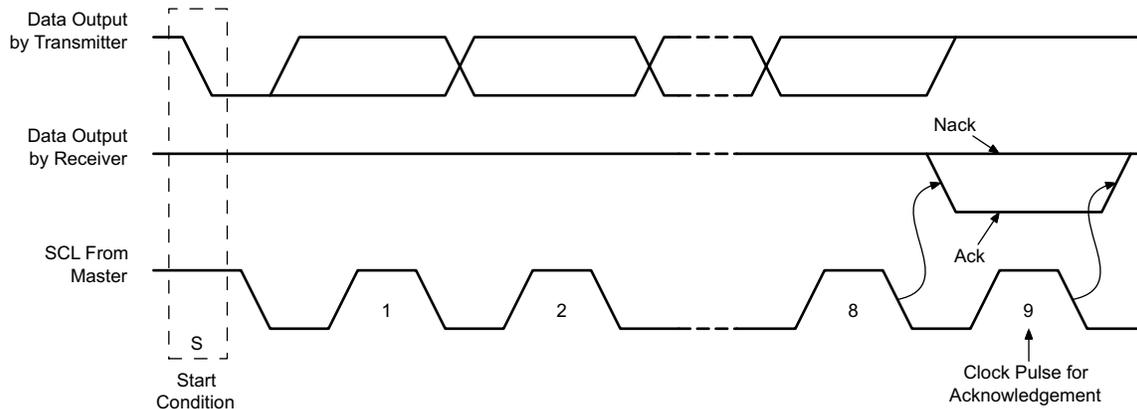
Figure 28. I<sup>2</sup>C Acknowledgment
