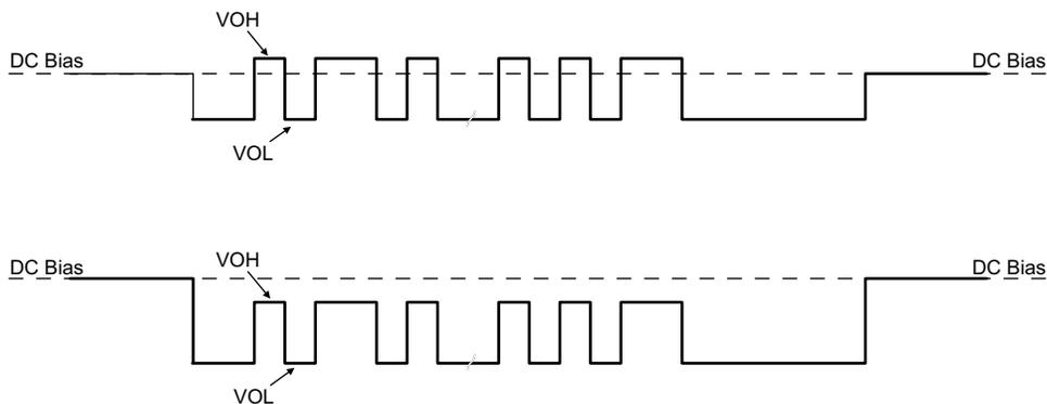
Figure 9. TX Driver Transmission with DC Bias
