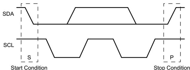
Figure 26. I<sup>2</sup>C Definition of Start and Stop Conditions
