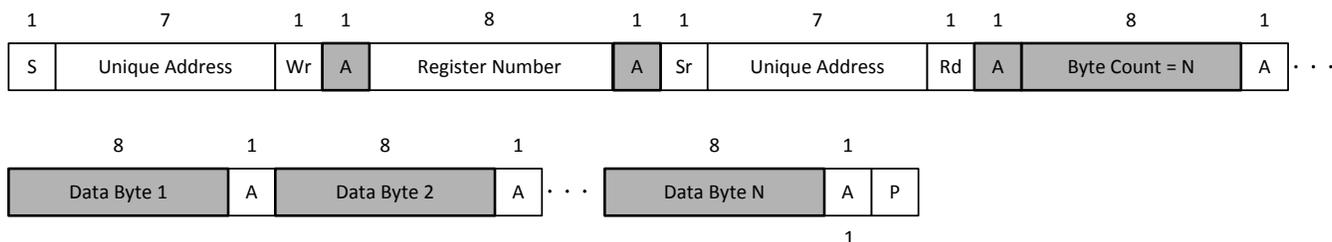
**Figure 30. I<sup>2</sup>C Unique Address Read Register Protocol**
