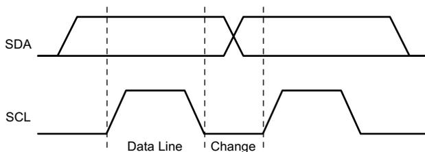
Figure 27. I<sup>2</sup>C Bit Transfer
