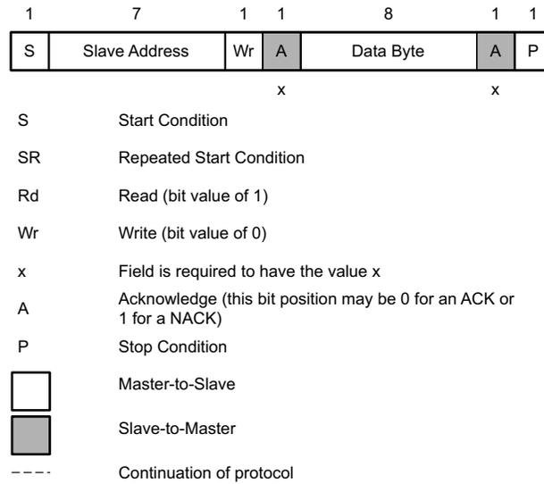
Figure 31. I<sup>2</sup>C Read/Write Protocol Key
