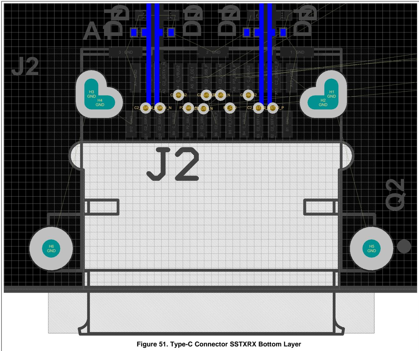
Figure 51. Type-C Connector SSTXRX Bottom Layer
