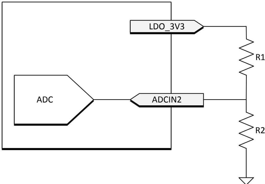
Figure 32. I<sup>2</sup>C Address Divider
