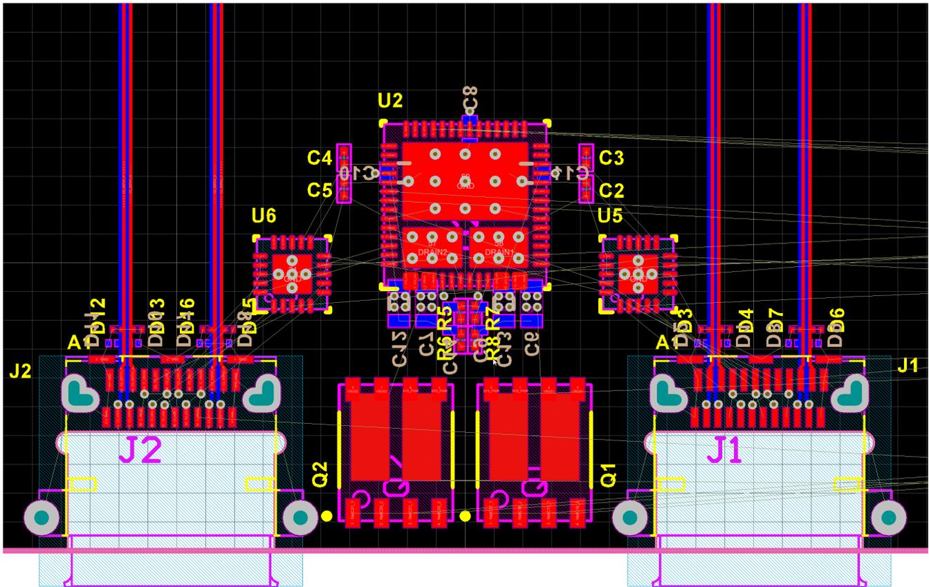
Figure 56. Protection Placement
