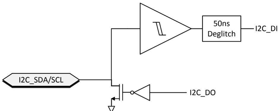
Figure 23. I<sup>2</sup>C Buffer
