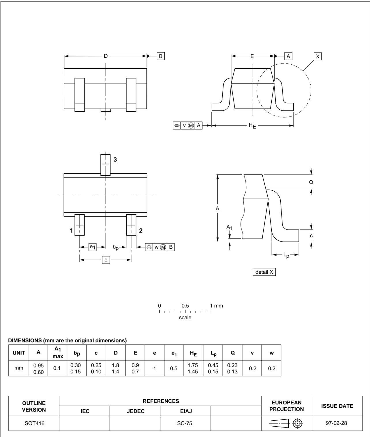
PNP resistor-equipped transistors;
