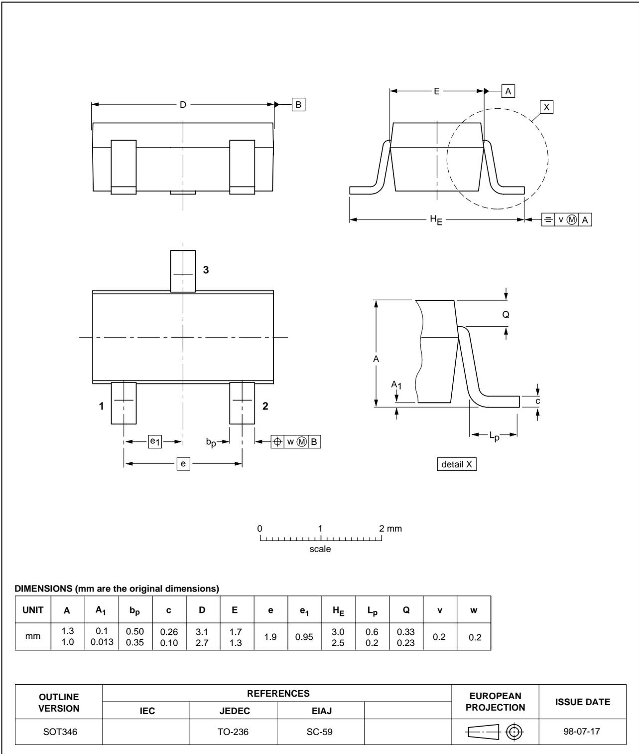
PNP resistor-equipped transistors;
