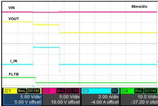
Figure 10. Over Current Protection, Thermal Shutdown (Latch-off)
