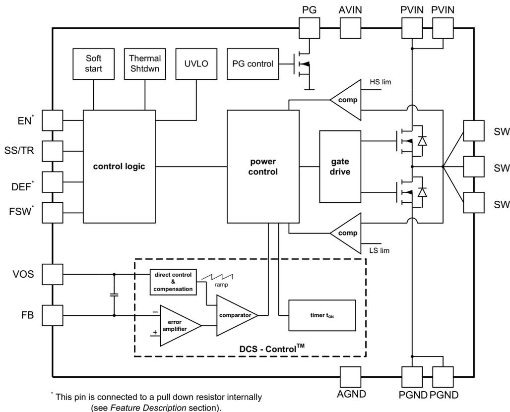
**Figure 5. TPS62130 and TPS62130A (Adjustable Output Voltage)**
