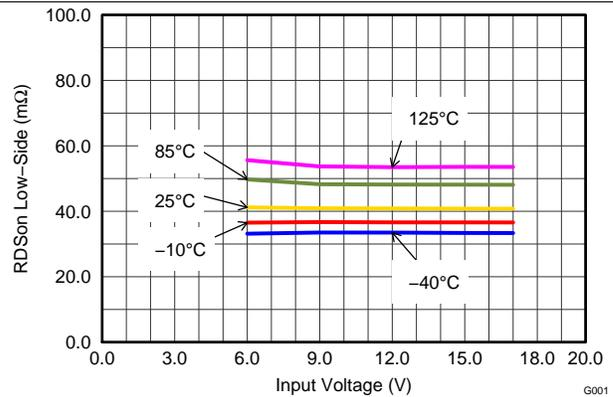
**Figure 4. Low-Side Switch Resistance**
