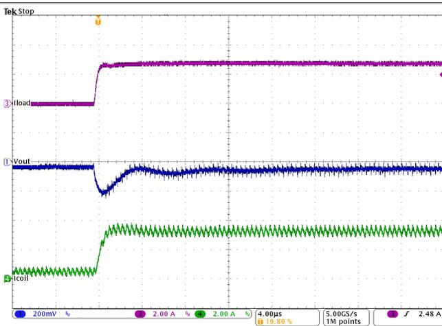
Figure 38. Load Transient Response of Figure 37, Rising Edge
