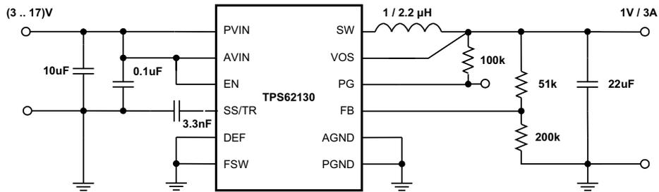
**Figure 55. 1V/3A Power Supply**
