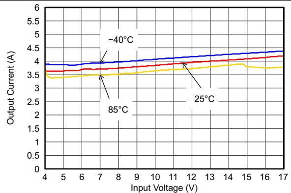
Figure 33. Maximum Output Current
