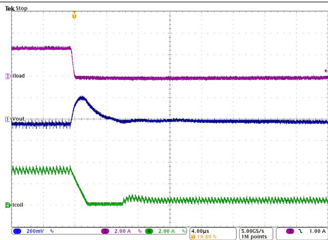
Figure 39. Load Transient Response of Figure 37, Falling Edge
