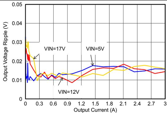
Figure 32. Output Voltage Ripple
