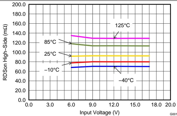
**Figure 3. High-Side Switch Resistance**
