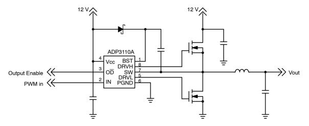
Figure 4. ADP3110A Example Circuit
