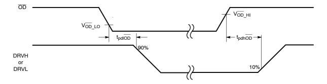
Figure 2. Output Disable Timing Diagram
