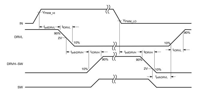
Figure 3. Nonoverlap Timing Diagram
