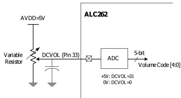
Figure 18. Volume Control by External Variable Resistor
