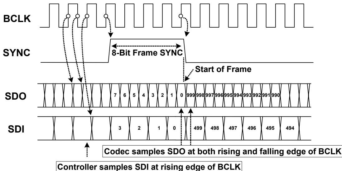
**Figure 5. Bit Timing**
