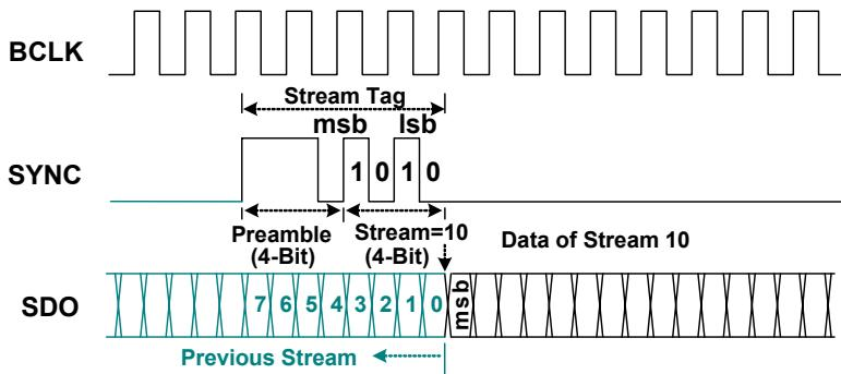
Figure 8. SDO Stream Tag is Indicated in SYNC
