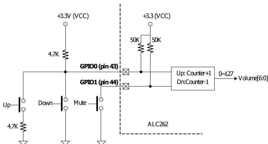
Figure 19. Volume Control via GPIO0 and GPIO1
