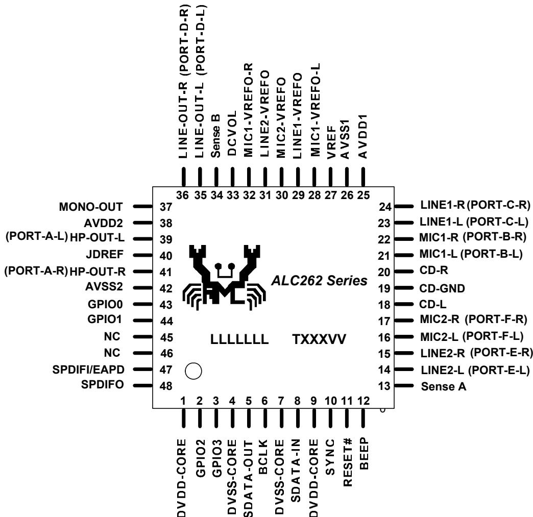
Figure 3. Pin Assignments
