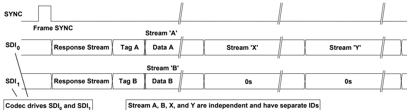
Figure 12. Codec Transmits Data Over Multiple SDIs
