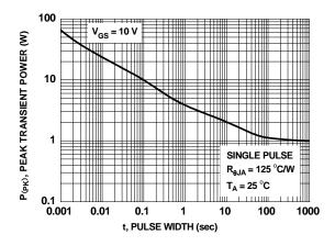
Figure 25. Single Pulse Maximum Power Dissipation
