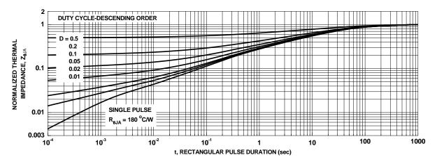
Figure 13. Junction-to-Ambient Transient Thermal Response Curve
