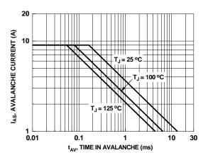
Figure 22. Unclamped Inductive Switching Capability
