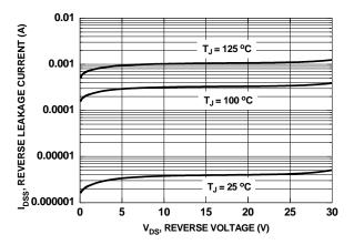
Figure 28. SyncFET body diode reverses leakage versus drain-source voltage
