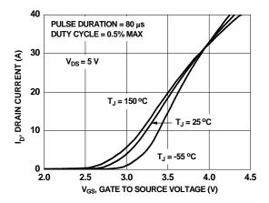
Figure 5. Transfer Characteristics
