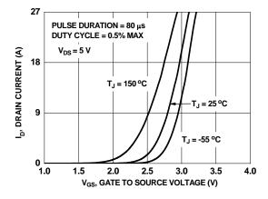
Figure 18. Transfer Characteristics
