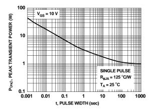
Figure 12. Single Pulse Maximum Power Dissipation
