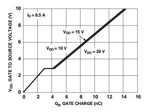
Figure 20. Gate Charge Characteristics
