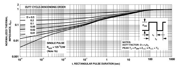
Figure 26. Junction-to-Ambient Transient Thermal Response Curve
