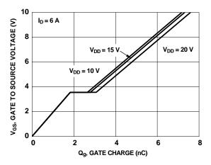
Figure 7. Gate Charge Characteristics
