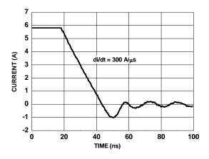
Figure 27. FDMC8200S SyncFET body diode reverse recovery characteristic
