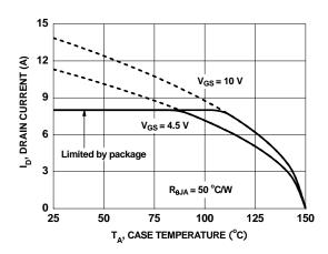
Figure 23. Maximum Continuous Drain Current vs Case Temperature
