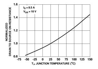
Figure 16. Normalized On-Resistance vs Junction Temperature
