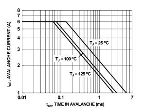
Figure 9. Unclamped Inductive Switching Capability
