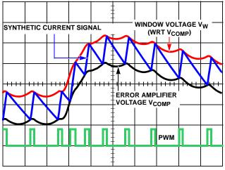
FIGURE 12. MODULATOR WAVEFORMS DURING LOAD TRANSIENT
