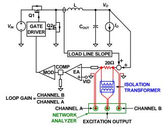
FIGURE 26. LOOP GAIN T1(s) MEASUREMENT SET-UP
