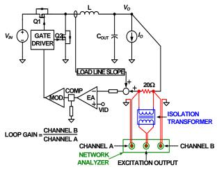
FIGURE 27. LOOP GAIN T2(s) MEASUREMENT SET-UP
