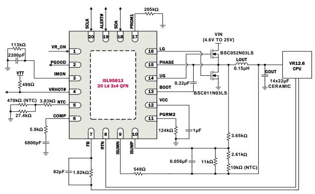
FIGURE 1. TYPICAL 40Amax, 12.6, APPLICATION DIAGRAM
