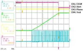
FIGURE 10. PS4 EXIT TO 1.6V, IO = 1A, SLEWRATE =  $53mV/\mu s$
