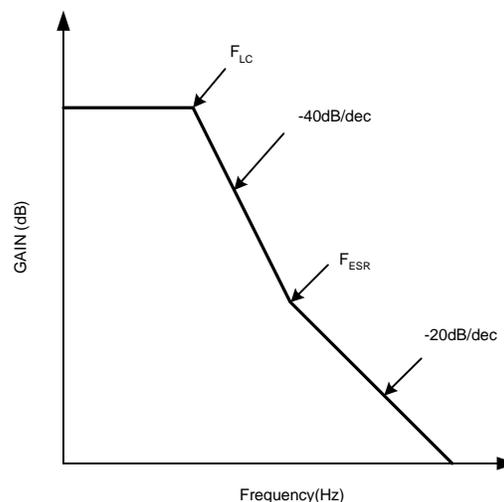
Figure 6. Frequency Resopnse of the LC Filters
