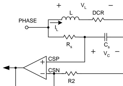
Figure 3. Illustration of Inductor Current Sensing Circuit
