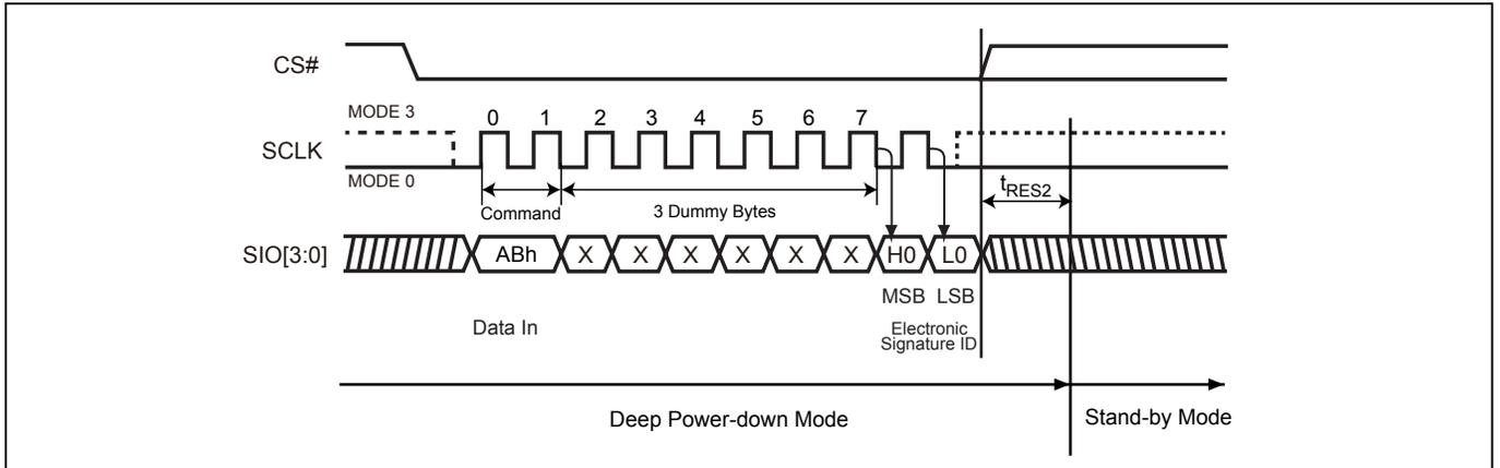
**Figure 15. Release from Deep Power-down (RDP) Sequence (SPI Mode)**
