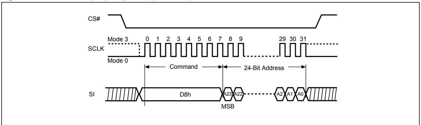
**Figure 43. Block Erase (BE) Sequence (QPI Mode)**
