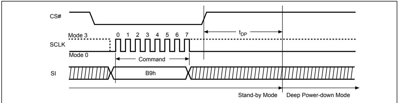
**Figure 50. Deep Power-down (DP) Sequence (QPI Mode)**
