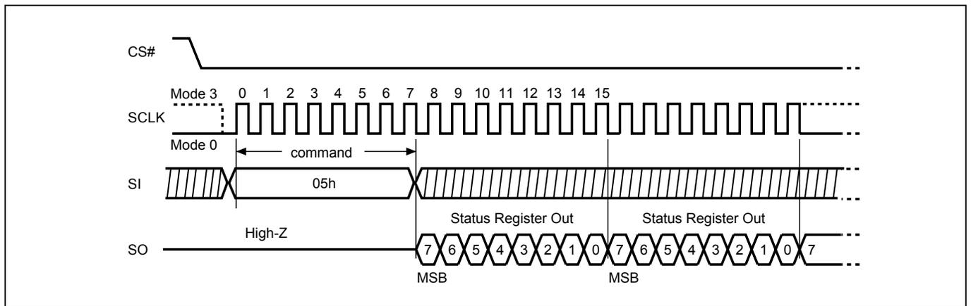
**Figure 19. Read Status Register (RDSR) Sequence (QPI Mode)**
