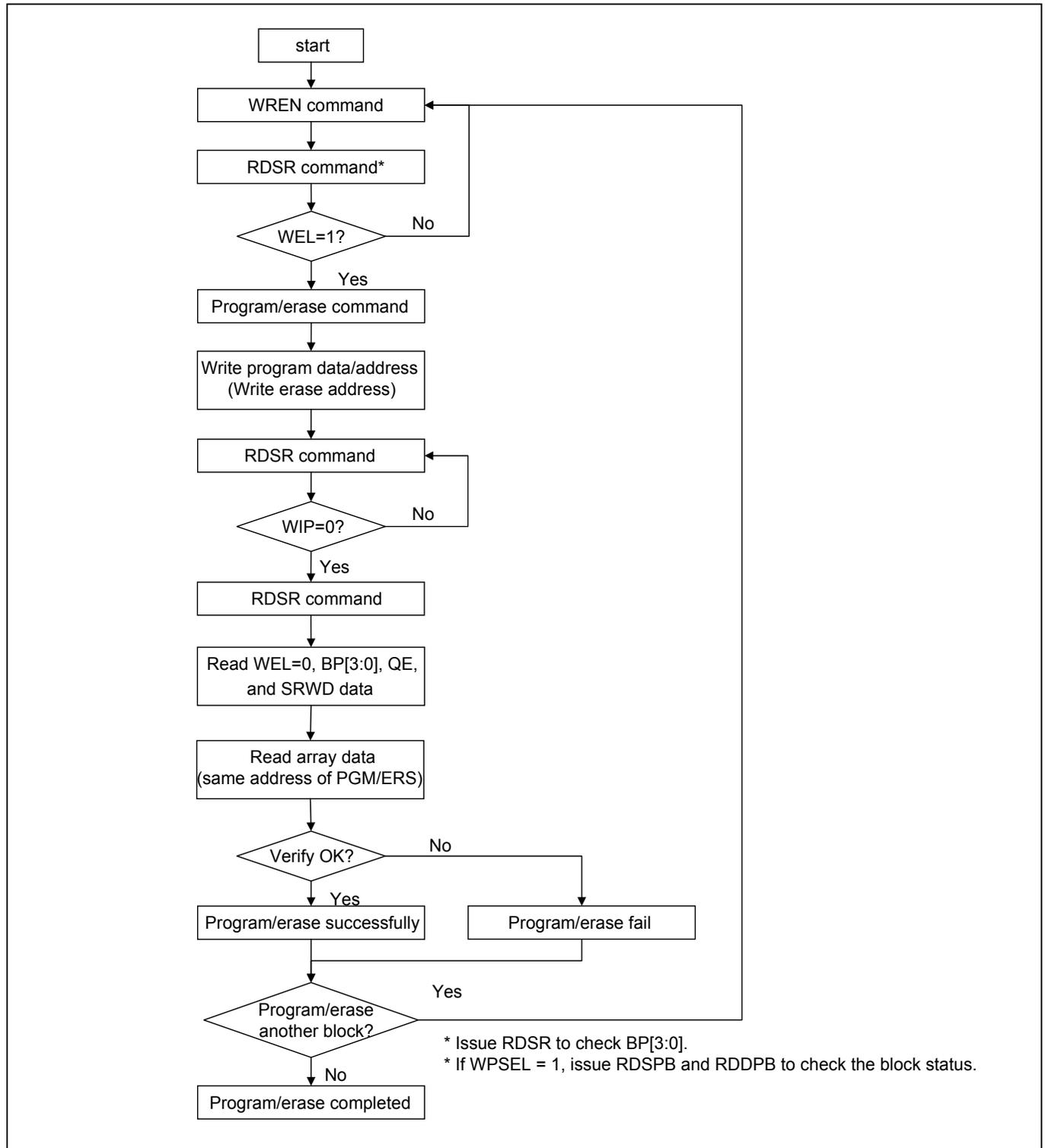
**Figure 23. Program/Erase flow without read array data (read P\_FAIL/E\_FAIL flag)**
