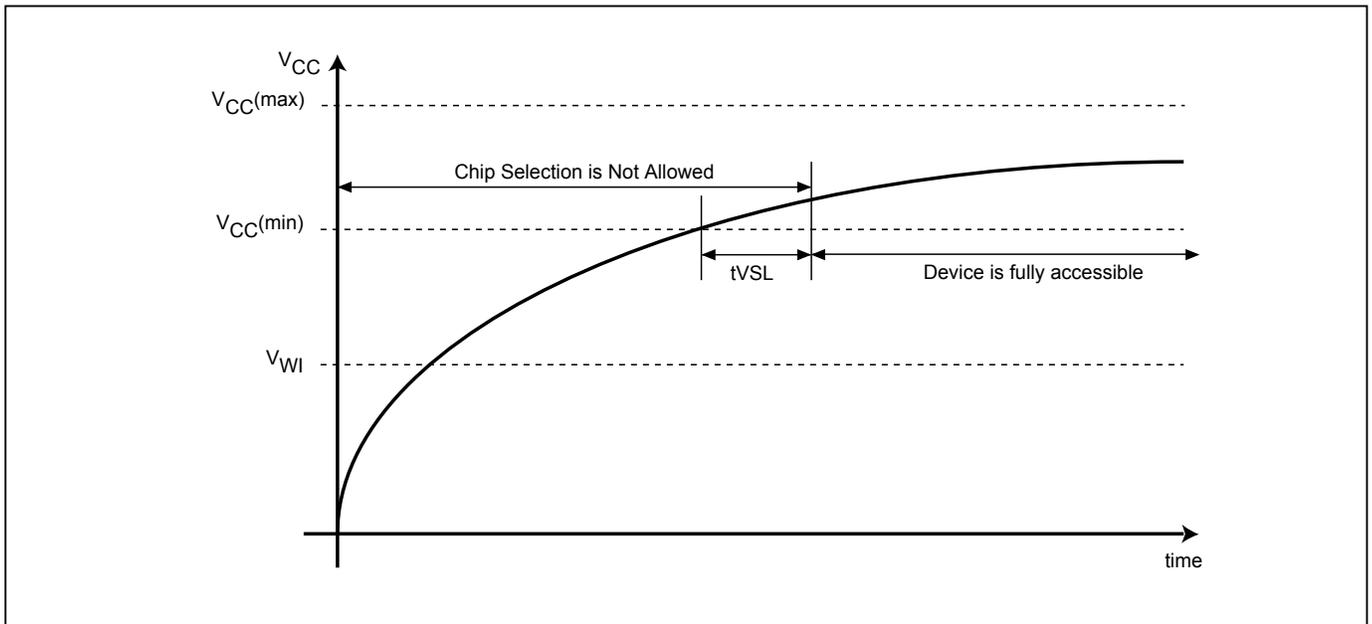
**Figure 80. Power Up/Down and Voltage Drop**
