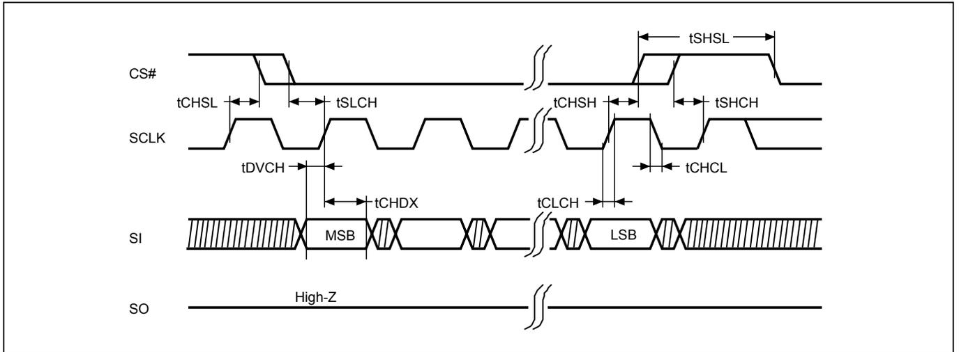
**Figure 3. Output Timing**
