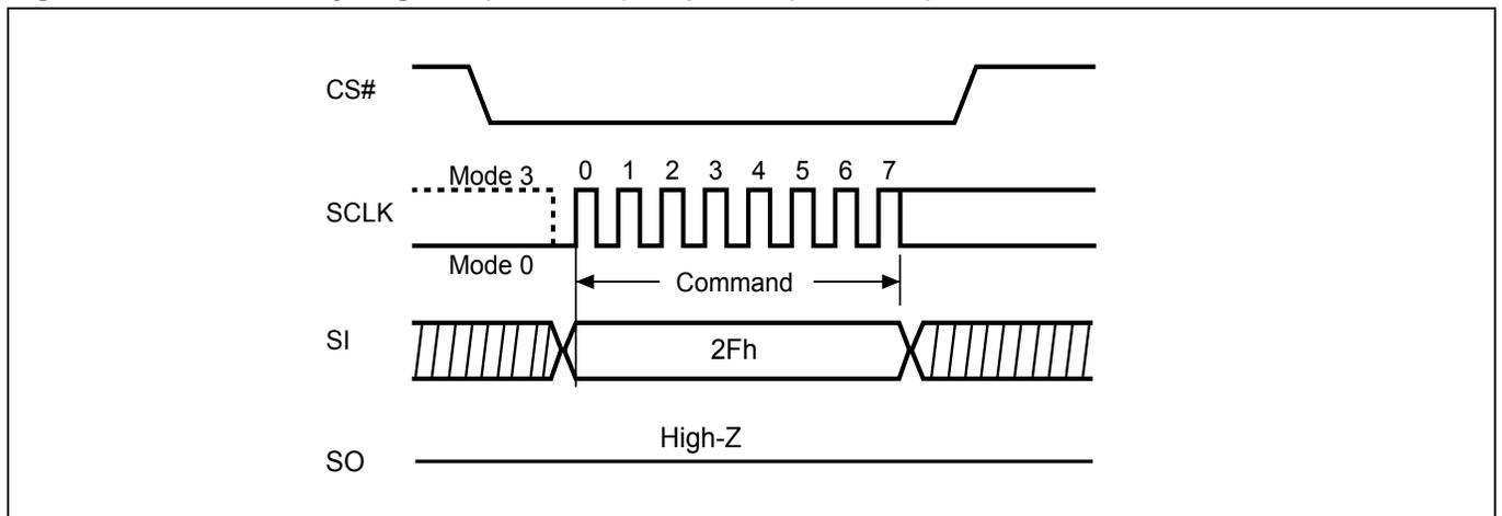
**Figure 52. Write Security Register (WRSCUR) Sequence (QPI Mode)**
