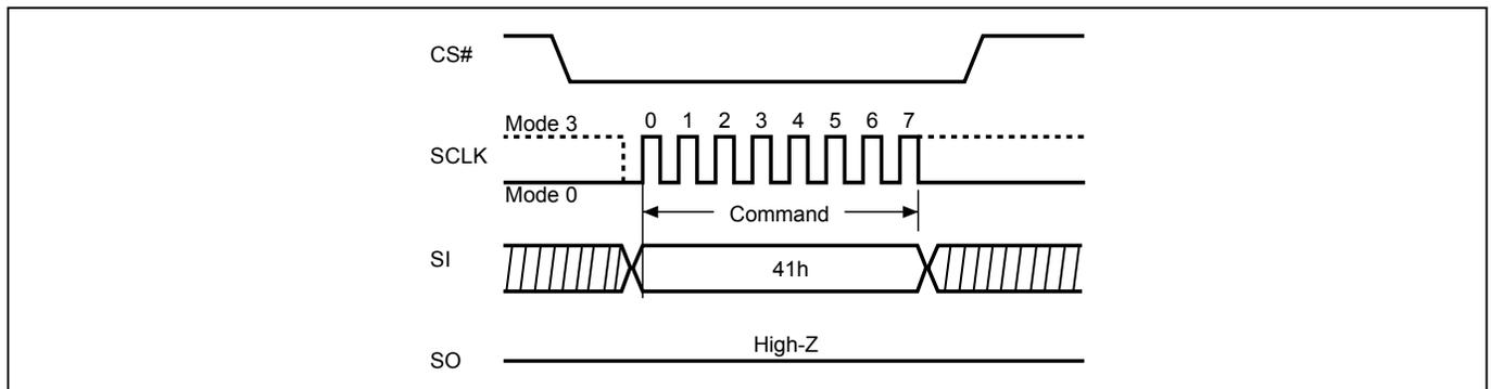
**Figure 11. Factory Mode Enable (FMEN) Sequence (QPI Mode)**
