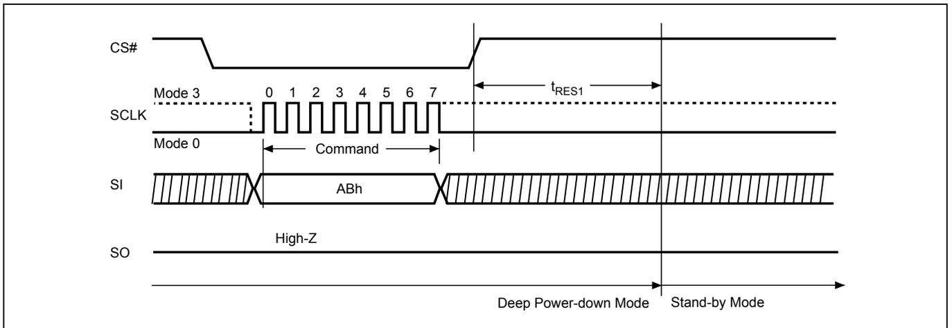
**Figure 16. Release from Deep Power-down (RDP) Sequence (QPI Mode)**
