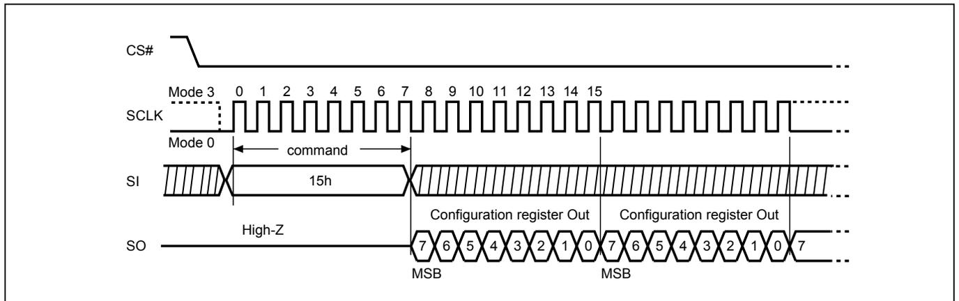
**Figure 21. Read Configuration Register (RDCR) Sequence (QPI Mode)**
