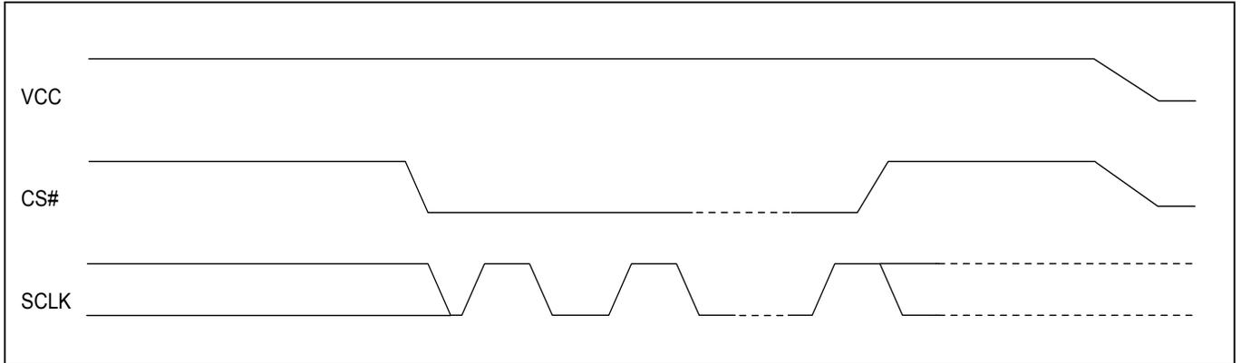
**Figure 79. Power-up Timing**
