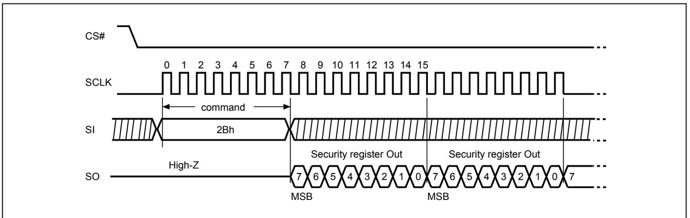
**Figure 54. Read Security Register (RDSCUR) Sequence (QPI Mode)**
