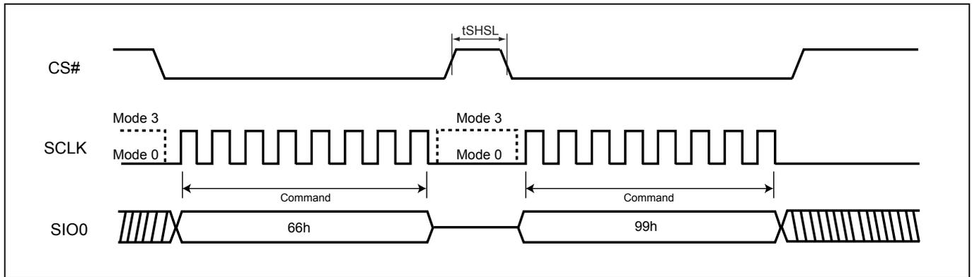
**Figure 70. Reset Sequence (QPI mode)**
