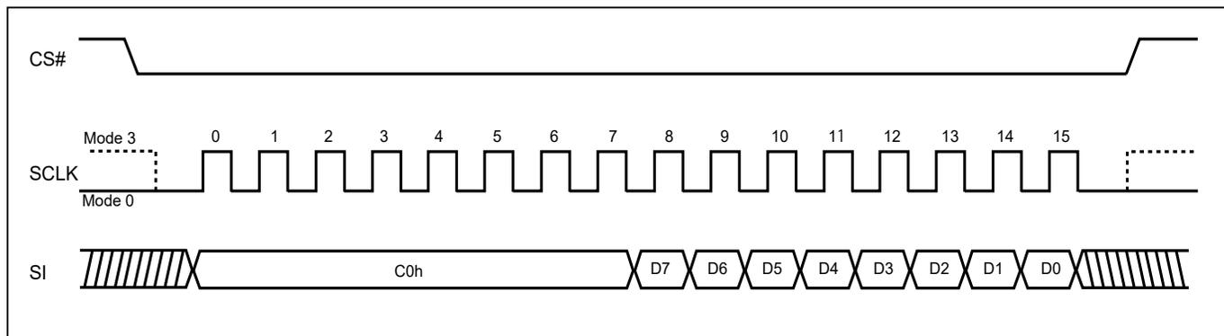
**Figure 35. Burst Read - QPI Mode**
