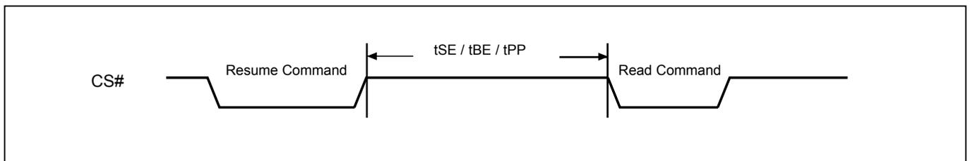
**Figure 67. Resume to Suspend Latency**
