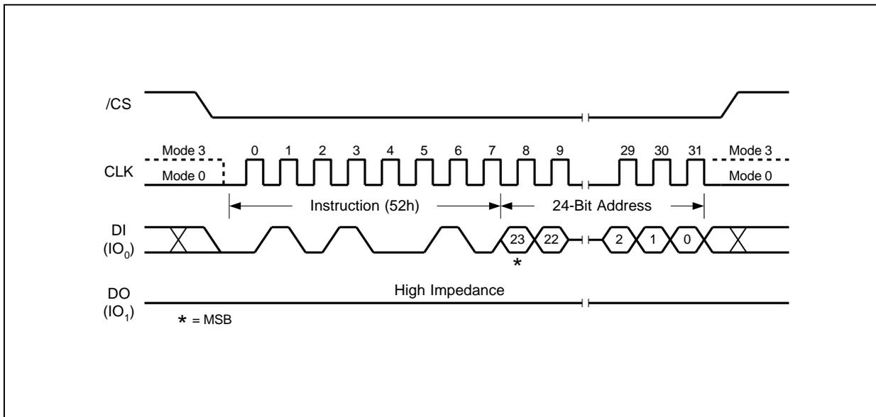
Figure 22. 32KB Block Erase Instruction Sequence Diagram
