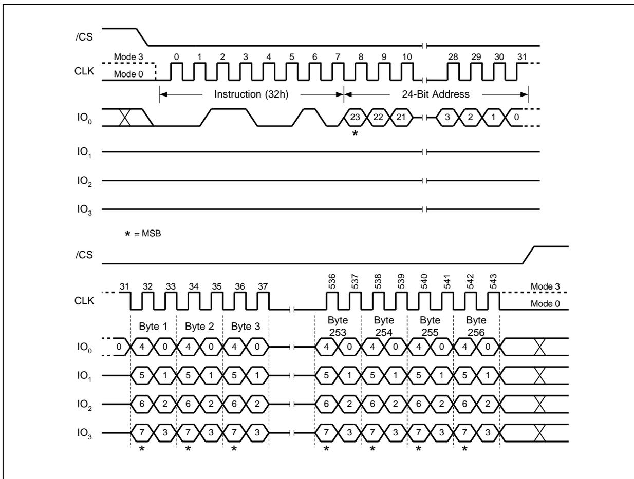
Figure 20. Quad Input Page Program Instruction Sequence Diagram
