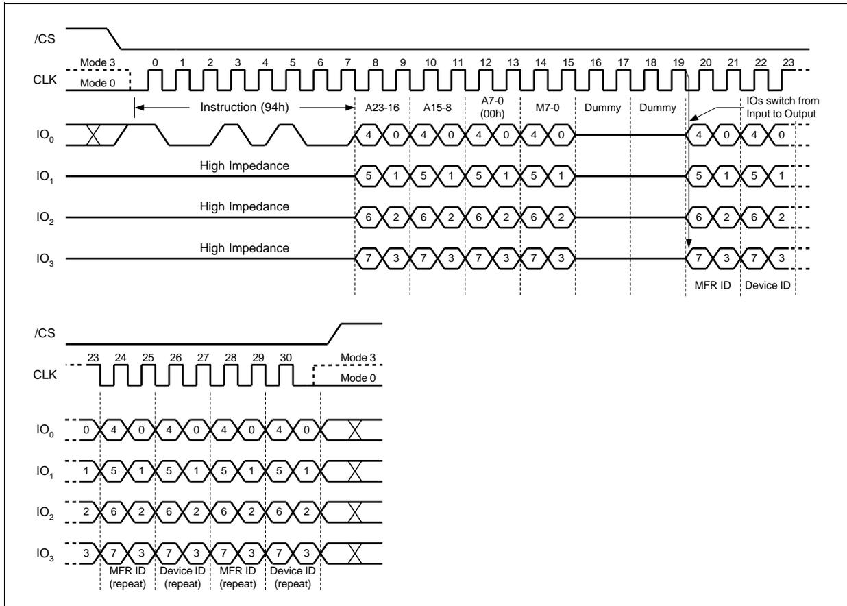
Figure 31. Read Manufacturer / Device ID Quad I/O Diagram
