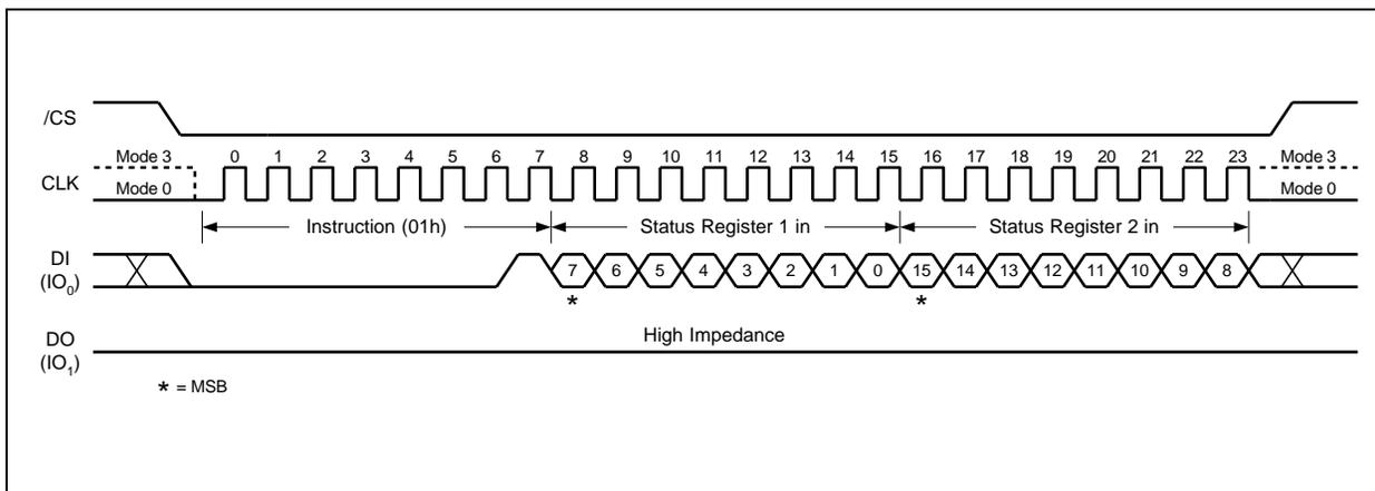
Figure 8. Write Status Register Instruction Sequence Diagram
