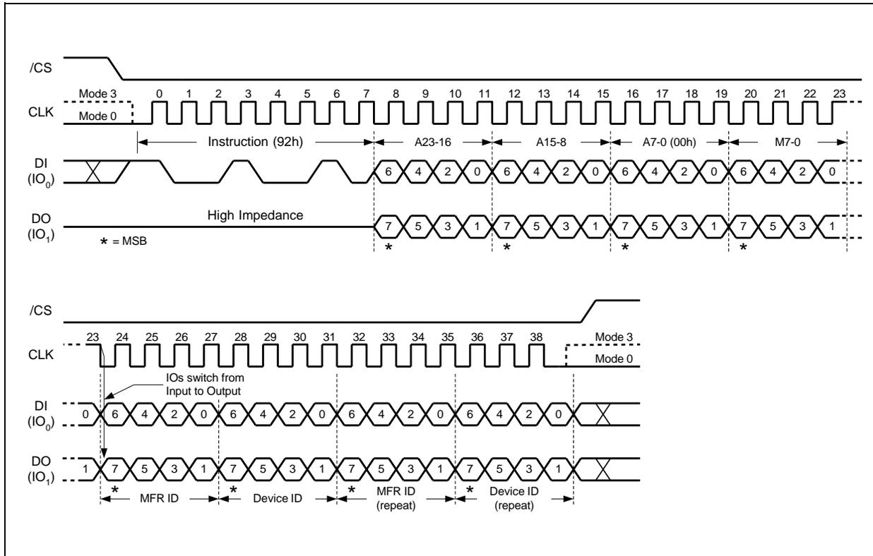
Figure 30. Read Manufacturer / Device ID Dual I/O Diagram
