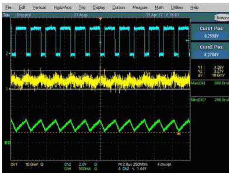
Figure 14. Ceramic 10 \mu F 0603 (X5R) (Good)
