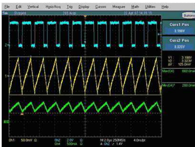
Figure 21. Electrolytic 100 \mu F (Ripple Too High)
