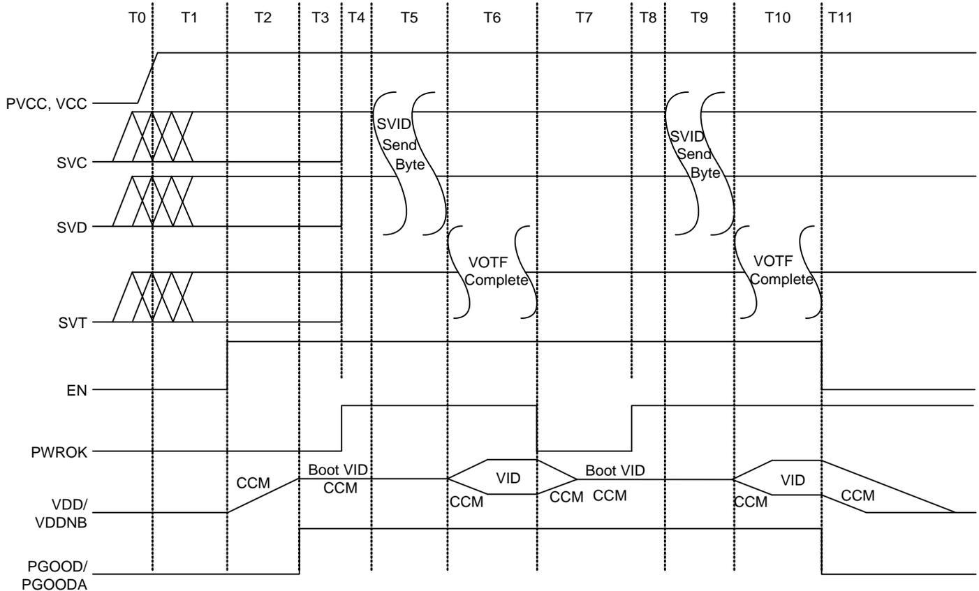
Figure 3. Simplified Sequence Timing Diagram
