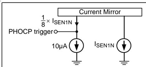
Figure 13. VDD Controller : Per-Phase OCP Setting
