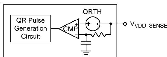
Figure 14. VDD Controller : Quick Response Triggering Circuit
