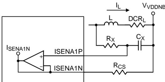
Figure 19. VDDNB Controller : Lossless Inductor Sensing
