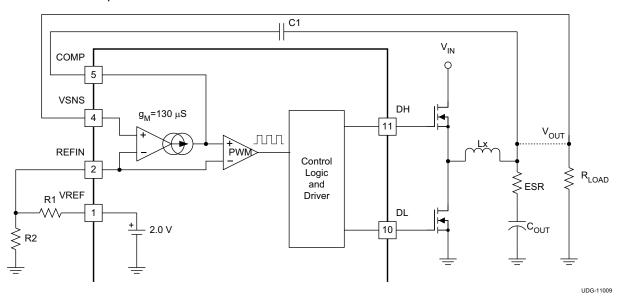
Figure 25. Simplified D-CAP™ Model
