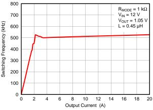
Figure 9. Switching Frequency vs Load Current
