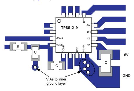
Figure 31. Case 1: COMP Pin Capacitance Connected to VSNS
