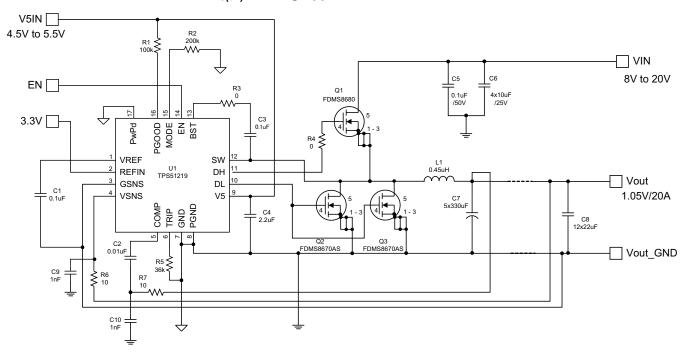
Figure 34. 1.05-V/20-A, D-CAP  $^{\text{TM}}$  400-kHz,  $R_{\text{DS(on)}}$  Sensing
