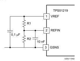
Figure 23. Voltage Reference Connections
