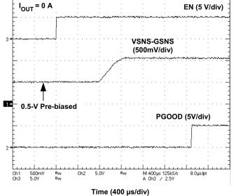
Figure 19. 1.05-V Startup Waveforms
