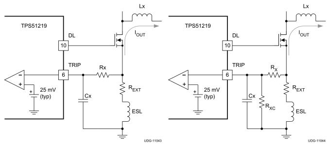
Figure 28. Resistor Sensing with Compensation
