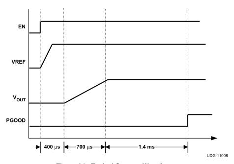
Figure 24. Typical Start-up Waveforms
