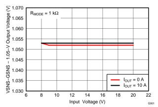
Figure 12. 1.05-V Output Line Regulation
