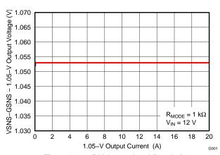
Figure 11. 1.05-V Output Load Regulation
