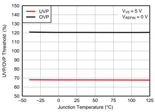
Figure 4. OVP/UVP Threshold vs Junction Temperature
