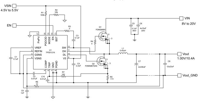
Figure 35. 1.00-V/10.4-A, D-CAP2™ 500-kHz, Resistor Sensing
