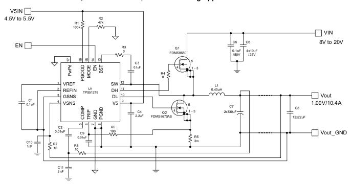
Figure 36. 1.00-V/10.4-A, D-CAP™ 400-kHz, Resistor Sensing
