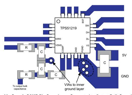
Figure 32. Case 2: COMP Pin Capacitance Connected to Output Bulk Capacitance
