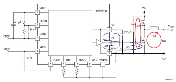
Figure 30. DC/DC Converter Ground System
