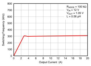
Figure 7. Switching Frequency vs Load Current
