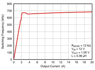
Figure 10. Switching Frequency vs Load Current
