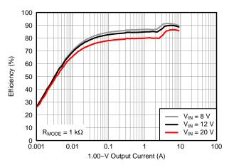
Figure 15. 1.00-V Output Line Regulation
