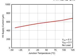
Figure 1. V5 Supply Current vs Junction Temperature
