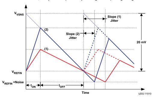
Figure 26. Ripple Voltage Slope and Jitter Performance
