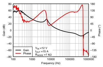
Figure 22. Bode Plot, V<sub>OUT</sub>=1.05 V
