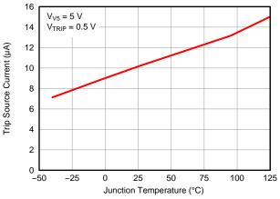
Figure 3. Current Sense Current vs Junction Temperature
