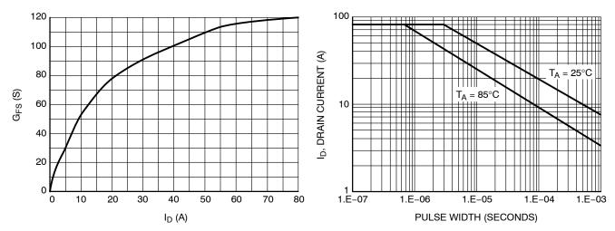
Figure 14. G<sub>FS</sub> vs. I<sub>D</sub> Figure 15. Avalanche Characteristics
