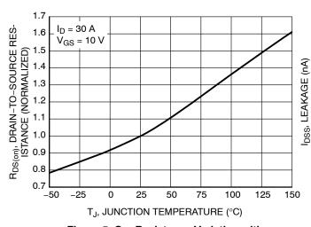
Figure 5. On–Resistance Variation with Temperature
