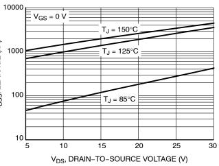
Figure 6. Drain-to-Source Leakage Current vs. Voltage
