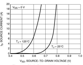
Figure 10. Diode Forward Voltage vs. Current
