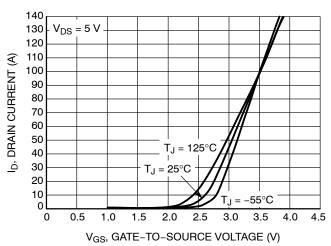
Figure 2. Transfer Characteristics
