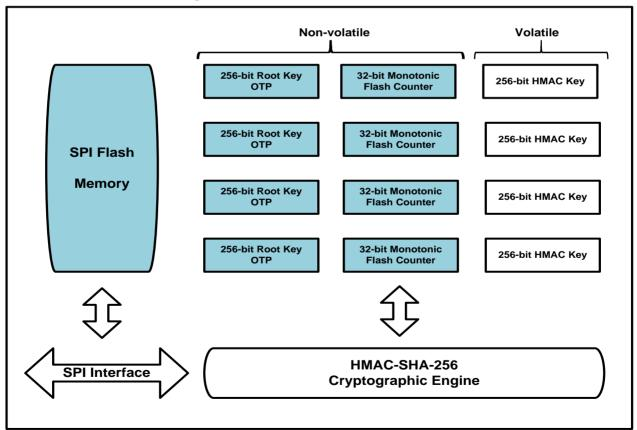
Figure 3. W74M12JW Functional Block Diagram
