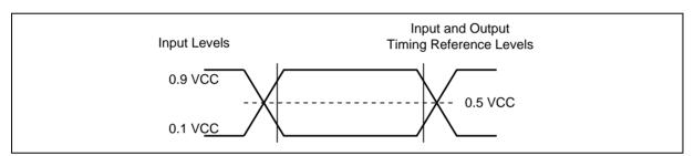
Figure 11. AC Measurement I/O Waveform
