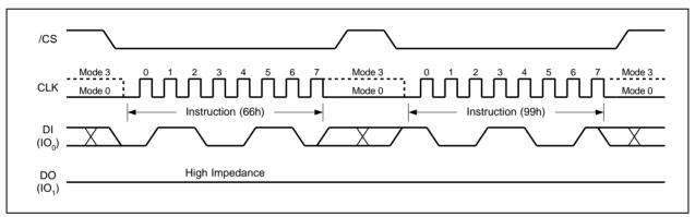
Figure 9. Enable Reset and Reset Instruction Sequence
