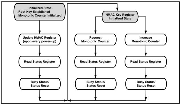
Figure 3b. W74M12JW Authentication Flash Operation Flow Diagram
