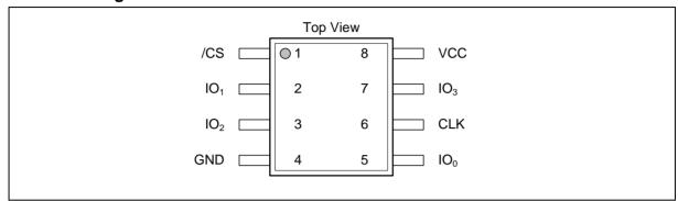
Figure 1a. W74M12JW Pin Assignments, 8-pin SOIC 208-mil (Package Code SS)
