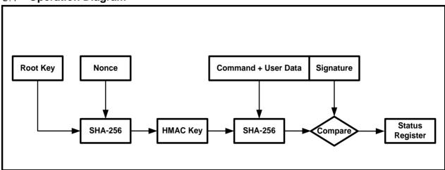
Figure 2. W74M12JW Operation Diagram
