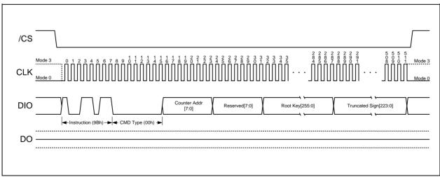
Figure 4. Write Root Key Register Instruction
