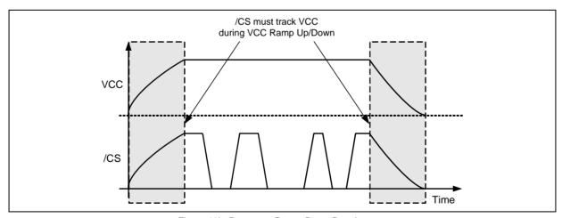
Figure 10b. Power-up, Power-Down Requirement
