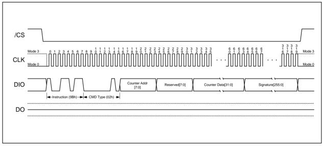
Figure 6. Increment Monotonic Counter Instruction
