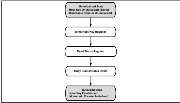
Figure 3a. W74M12JW Initialization Flow Diagram
