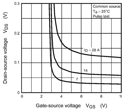
**Fig. 8.4  $V_{DS} - V_{GS}$**
