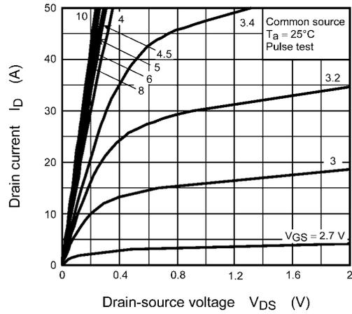
**Fig. 8.2  $I_D - V_{DS}$**
