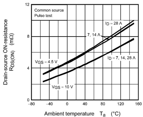
**Fig. 8.6  $R_{DS(ON)} - T_a$**
