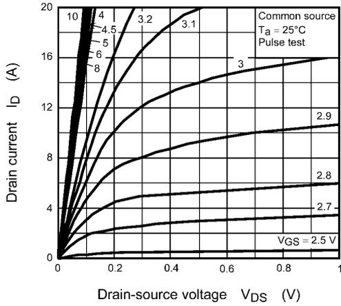
**Fig. 8.1  $I_D - V_{DS}$**
