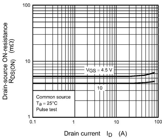
**Fig. 8.5  $R_{DS(ON)} - I_D$**
