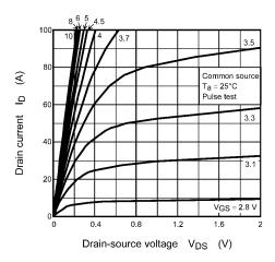
Fig. 8.2  $I_D - V_{DS}$
