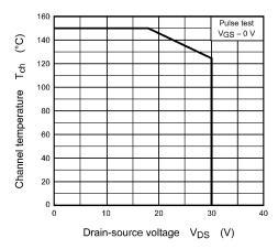
Fig. 8.17 T<sub>ch</sub>-V<sub>DS</sub> (Guaranteed Maximum)
