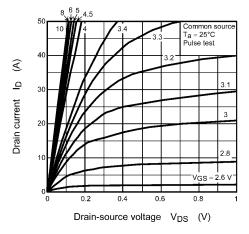
Fig. 8.1  $I_D - V_{DS}$
