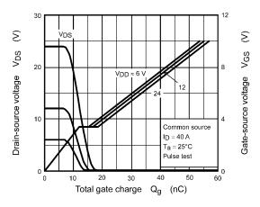
Fig. 8.10 Dynamic Input/Output Characteristics
