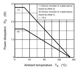
Fig. 8.11 P<sub>D</sub> - T<sub>a</sub> (Guaranteed Maximum)
