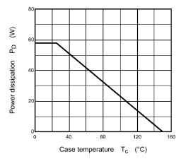
Fig. 8.12 P<sub>D</sub> - T<sub>c</sub> (Guaranteed Maximum)
