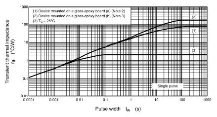
Fig. 8.13 r<sub>th</sub> - t<sub>w</sub> (Guaranteed Maximum)
