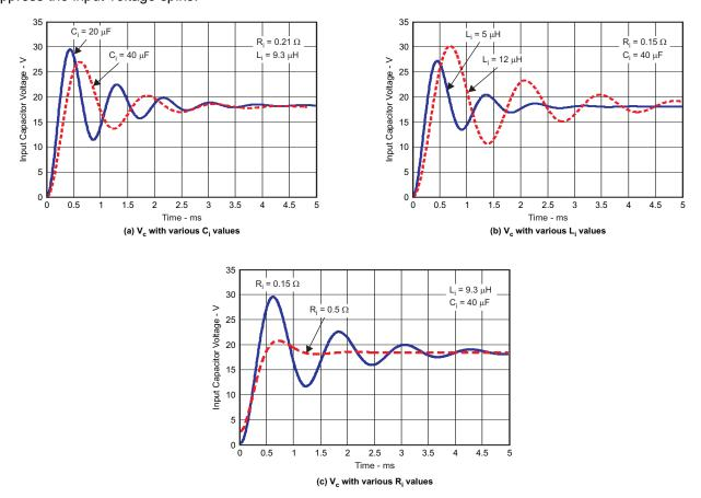
Figure 39. Parametric Study of the Input Voltage
