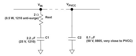
Figure 40. Recommended Input Filter Design
