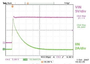
Figure 41. Adapter DC Side Hot Plug-in Test Waveforms
