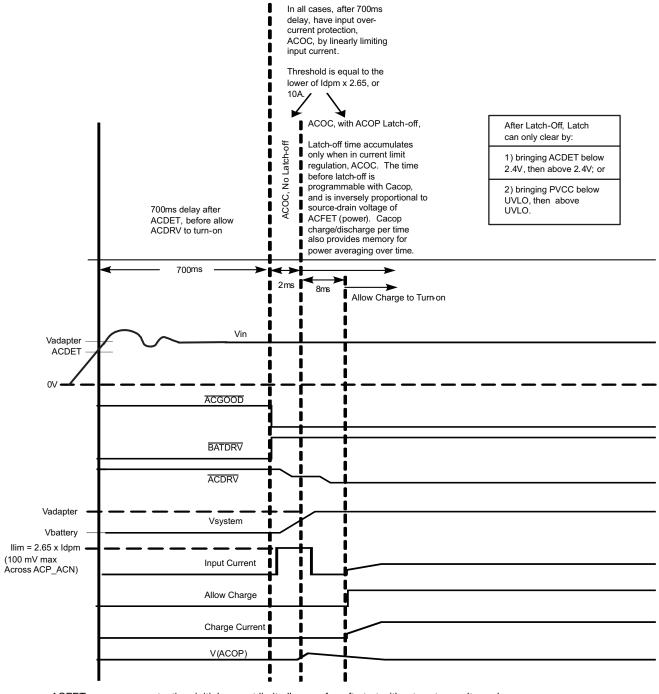
ACFET overpower protection; initial current limit allows safe soft-start without system voltage droop.
