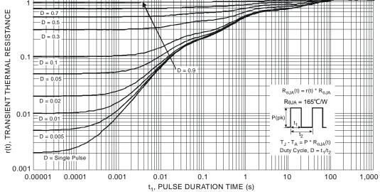
Fig. 11 Transient Thermal Response
