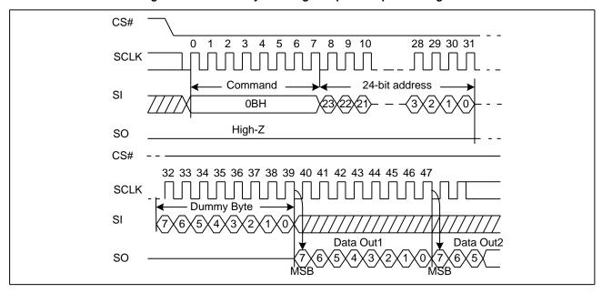
Figure 7. Read Data Bytes at Higher Speed Sequence Diagram
