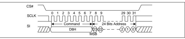
Figure 22. 64KB Block Erase Sequence Diagram
