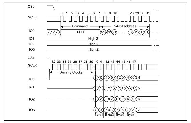
Figure 9. Quad Output Fast Read Sequence Diagram
