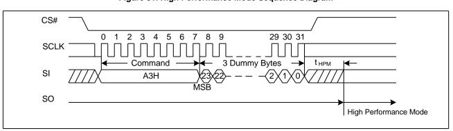
Figure 31. High Performance Mode Sequence Diagram
