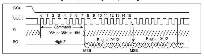
Figure 4. Read Status Register Sequence Diagram
