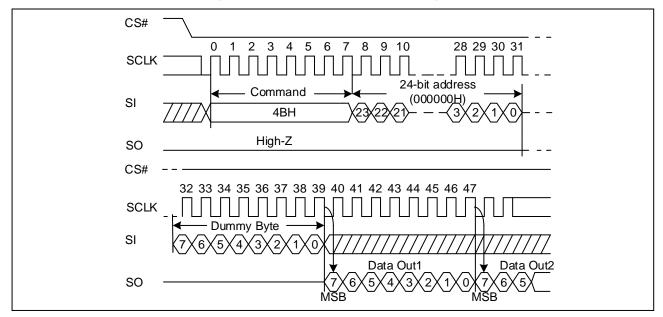
Figure 32. Read Unique ID Sequence Diagram
