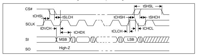
Figure 43. Output Timing
