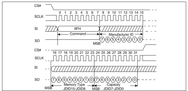
Figure 30. Read Identification ID Sequence Diagram
