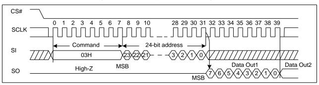
Figure 6. Read Data Bytes Sequence Diagram
