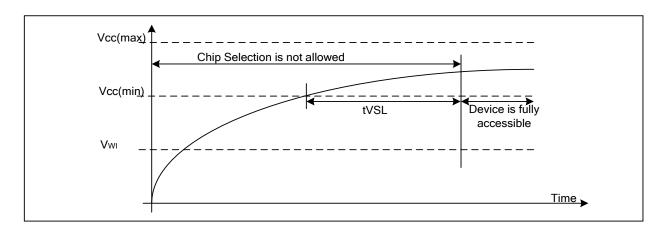
Table6. Power-Up Timing and Write Inhibit Threshold
