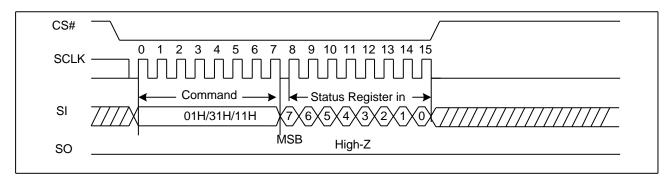
Figure 5. Write Status Register Sequence Diagram
