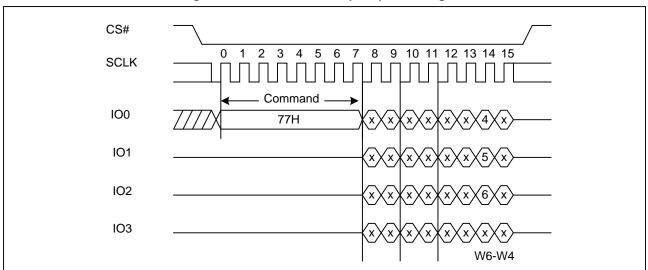
Figure 16. Set Burst with Wrap Sequence Diagram
