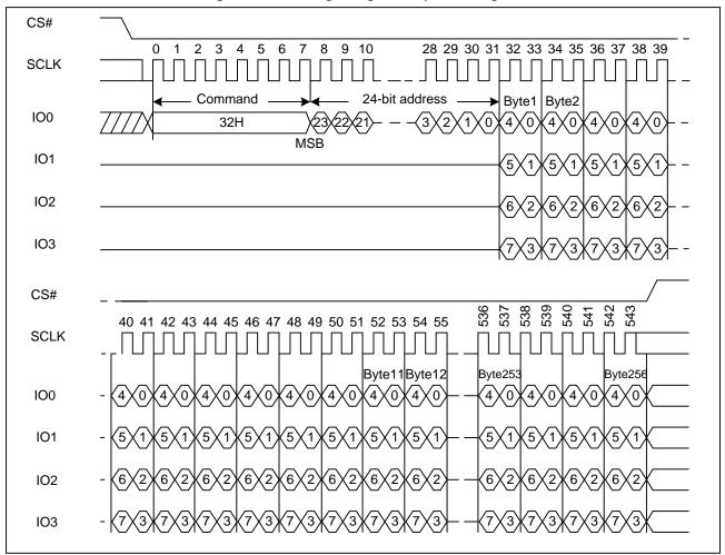
Figure 18. Quad Page Program Sequence Diagram
