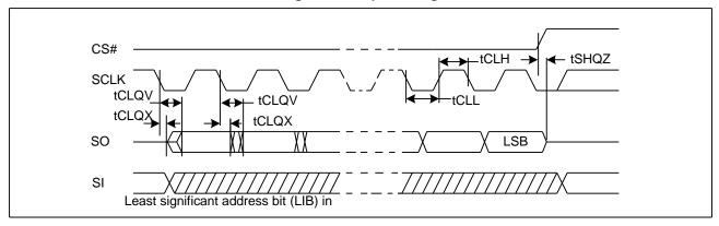
Figure 44. Resume to Suspend Timing
