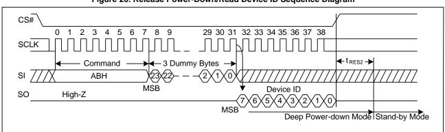
Figure 26. Release Power-Down/Read Device ID Sequence Diagram
