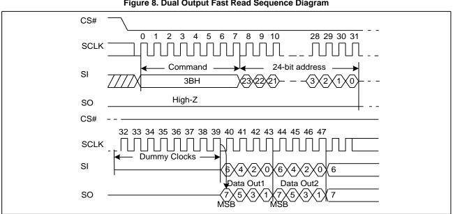
Figure 8. Dual Output Fast Read Sequence Diagram
