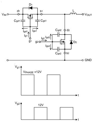
Figure 1. Equivalent Circuit and Associated Waveforms
