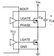
Figure 2. Part of Bootstrap Circuit of RT9611A/B
