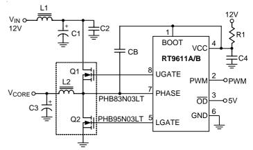
Figure 6. Synchronous Buck Converter Circuit
