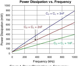
Figure 4. Power Dissipation vs. Frequency
