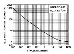
Figure 25. Single Pulse Maximum Power Dissipation
