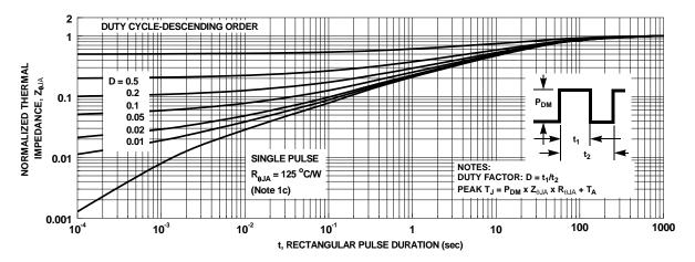
Figure 13. Junction-to-Ambient Transient Thermal Response Curve
