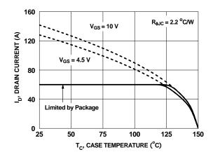
Figure 23. Maximun Continuous Drain Current vs Case Temperature
