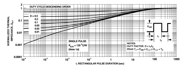
Figure 26. Junction-to-Ambient Transient Thermal Response Curve
