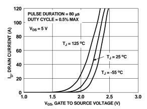
Figure 18. Transfer Characteristics
