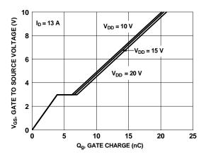
Figure 7. Gate Charge Characteristics
