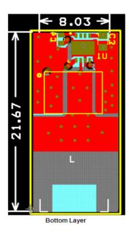
Figure 31. Recommended PCB Layout
