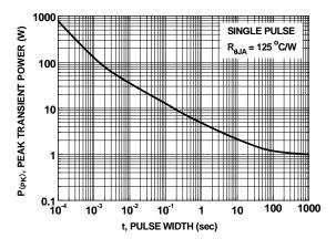
Figure 12. Single Pulse Maximum Power Dissipation
