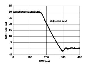
Figure 27. FDMS3660S SyncFET body diode reverse recovery characteristic
