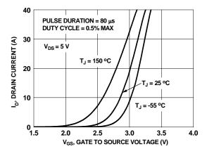
Figure 5. Transfer Characteristics
