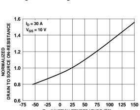
Figure 16. Normalized On-Resistance vs Junction Temperature
