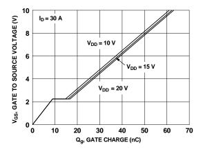
Figure 20. Gate Charge Characteristics
