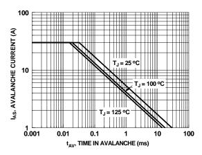
Figure 9. Unclamped Inductive Switching Capability
