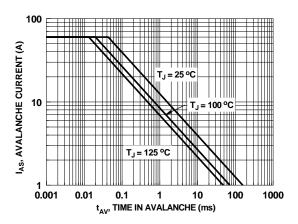
Figure 22. Unclamped Inductive Switching Capability
