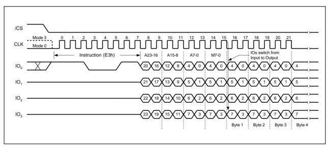
Figure 27a. Octal Word Read Quad I/O Instruction (Initial instruction or previous M5-4 ≠ 10, SPI Mode only)
