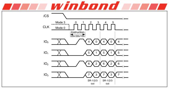
Figure 8b. Read Status Register Instruction (QPI Mode)
