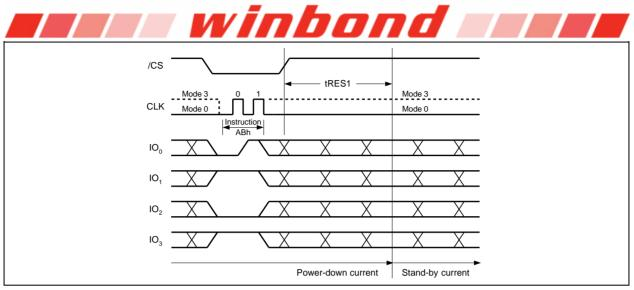
Figure 38b. Release Power-down Instruction (QPI Mode)
