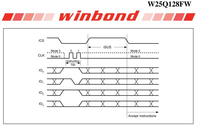
Figure 35b. Erase/Program Suspend Instruction (QPI Mode)
