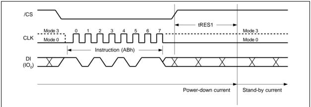
Figure 38a. Release Power-down Instruction (SPI Mode)
