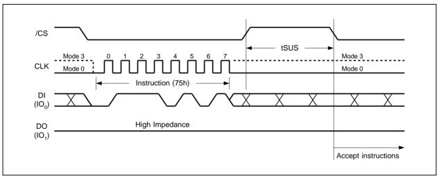
Figure 35a. Erase/Program Suspend Instruction (SPI Mode)
