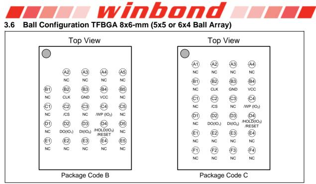
Figure 1d. W25Q128FW Ball Assignments, 24-ball TFBGA 8x6-mm (Package Code B & C)
