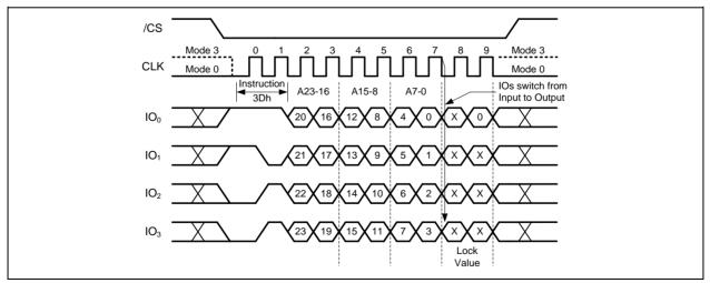
Figure 53b. Read Block Lock Instruction (QPI Mode)
