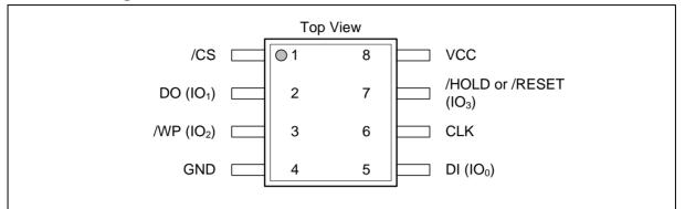
Figure 1a. W25Q128FW Pin Assignments, 8-pin SOIC 208-mil (Package Code S)
