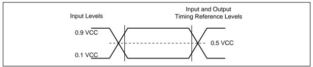
Figure 58. AC Measurement I/O Waveform
