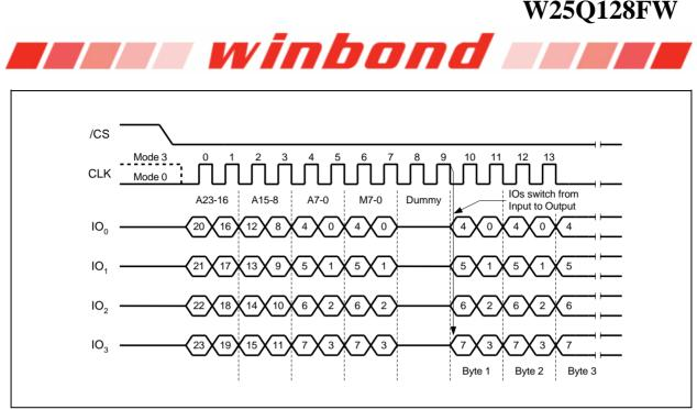
Figure 26b. Word Read Quad I/O Instruction (Previous instruction set M5-4 = 10, SPI Mode only)
