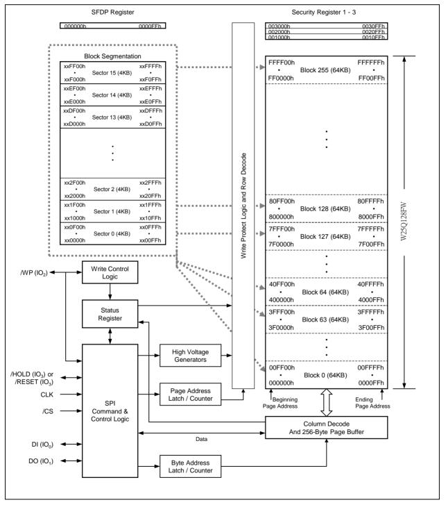
Figure 2. W25Q128FW Serial Flash Memory Block Diagram
