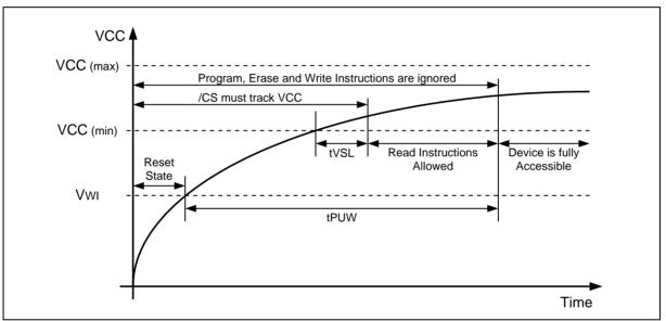
Figure 57. Power-up Timing and Voltage Levels
