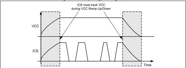
Figure 57a. Power-up, Power-Down Requirement
