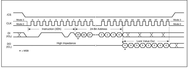
Figure 53a. Read Block Lock Instruction (SPI Mode)
