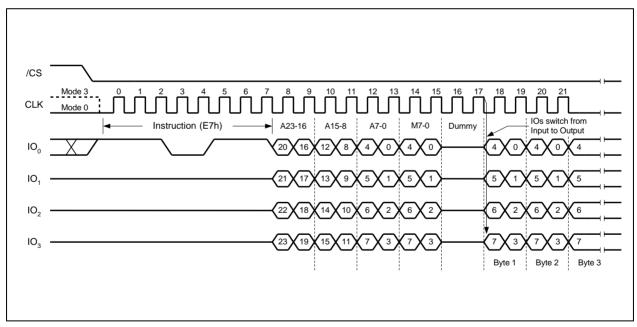
Figure 26a. Word Read Quad I/O Instruction (Initial instruction or previous  $M5-4 \neq 10$ , SPI Mode only)
