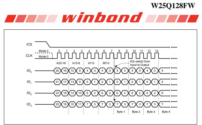
Figure 27b. Octal Word Read Quad I/O Instruction (Previous instruction set M5-4 = 10, SPI Mode only)
