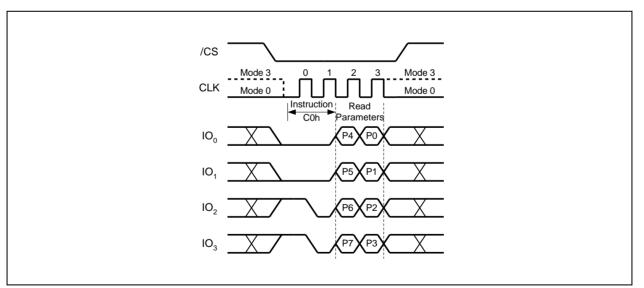
Figure 47. Set Read Parameters Instruction (QPI Mode only)
