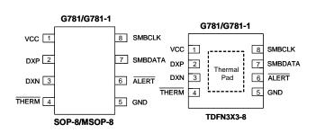
Note: Recommend connecting the Thermal Pad to the GND or let it keep floating.
