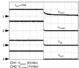
CH1: V<sub>5VCC</sub> (5V/div) CH2: V<sub>COMP</sub> (1V/div) CH3: V<sub>SS</sub> (5V/div) CH4: V<sub>OUT</sub> (1V/div) Time: 5ms/div
