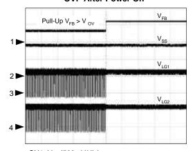
$\begin{array}{l} \text{CH1: V}_{\text{FB}} \text{ (500mV/div)} \\ \text{CH2: V}_{\text{SS}} \text{ (2V/div)} \\ \text{CH3: V}_{\text{LG1}} \text{ (10V/div)} \\ \text{CH4: V}_{\text{LG2}} \text{ (10V/div)} \\ \text{Time: 100} \text{ \mus/div} \end{array}$
