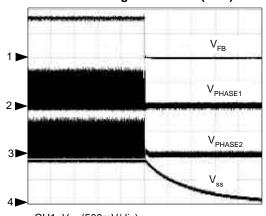
CH1:  $V_{FB}$  (500mV/div) CH2:  $V_{PHASE1}$  (10V/div) CH3:  $V_{PHASE2}$  (10V/div) CH4:  $V_{SS}$  (2V/div) Time: 500 $\mu$ s/div
