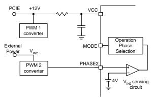
Figure 2.  $V_{IN2}$  Sensing Circuit
