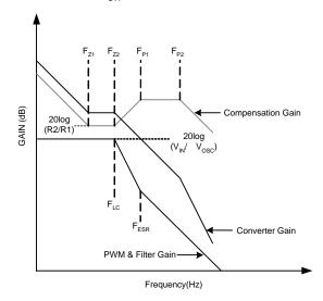
Figure 9. Converter Gain and Frequency
