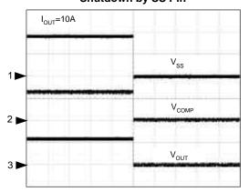
$\begin{array}{l} \text{CH1: V}_{\text{SS}} \left(2\text{V/div}\right) \\ \text{CH2: V}_{\text{COMP}} \left(1\text{V/div}\right) \\ \text{CH3: V}_{\text{OUT}} \left(1\text{V/div}\right) \\ \text{Time: 10ms/div} \end{array}$
