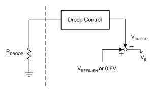
Figure 4. Illustration of Droop Setting Function
