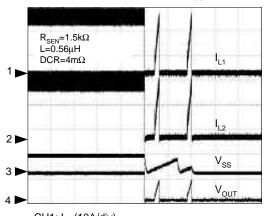
$\begin{array}{l} \text{CH1: I}_{\text{L1}}\left(10\text{A/div}\right) \\ \text{CH2: I}_{\text{L2}}\left(10\text{A/div}\right) \\ \text{CH3: V}_{\text{SS}}\left(5\text{V/div}\right) \\ \text{CH4: V}_{\text{OUT}}\left(1\text{V/div}\right) \\ \text{Time: 5ms/div} \end{array}$
