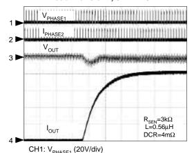
$\begin{array}{l} \text{CH1: V}_{\text{PHASE1}} \left( 20\text{V/div} \right) \\ \text{CH2: I}_{\text{PHASE2}} \left( 20\text{A/div} \right) \\ \text{CH3: V}_{\text{OUT}} \left( \text{AC, 200mV/div} \right) \\ \text{CH4: I}_{\text{OUT}} \left( 10\text{A/div} \right) \\ \text{Time: 20} \mu \text{s/div} \end{array}$
