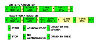
FIGURE 24. SMBus READ AND WRITE PROTOCOL
