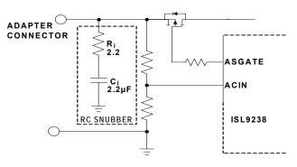
FIGURE 34. ADAPTER INPUT RC SNUBBER CIRCUIT
