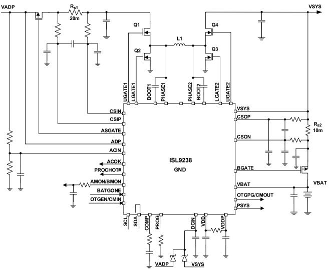
FIGURE 3. SIMPLIFIED APPLICATION DIAGRAM
