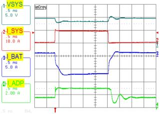
FIGURE 13. BUCK-BOOST MODE, CHARGING CURRENT LOOP TO ADAPTER CURRENT LOOP TRANSITION.  $V_{ADP} = 12V$ , MAXSYSTEMVOLTAGE = 12.576V,  $V_{BAT} = 11V$ , SYSTEM LOAD 1A TO 10A STEP, ADAPTERCURRENTLIMIT = 3A, CHARGECURRENT = 1A
