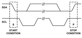
FIGURE 22. START AND STOP WAVEFORMS
