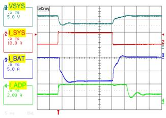
FIGURE 10. BOOST MODE, OUTPUT VOLTAGE LOOP TO ADAPTER CURRENT LOOP TRANSITION.  $V_{ADP} = 5V$ , MAXSYSTEMVOLTAGE = 12.576V,  $V_{BAT} = 11V$ , SYSTEM LOAD 0.5A TO 10A STEP, ADAPTERCURRENTLIMIT = 3A, CHARGECURRENT = 0A
