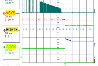
FIGURE 7. ADAPTER REMOVAL, V<sub>ADP</sub> = 20V, V<sub>BAT</sub> = 11V, CHARGECURRENT = 0A
