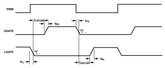
FIGURE 4. GATE DRIVER TIMING DIAGRAM
