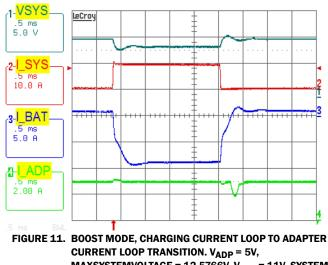
CURRENT LOOP TRANSITION.  $V_{ADP} = 5V$ , MAXSYSTEMVOLTAGE = 12.5766V,  $V_{BAT} = 11V$ , SYSTEM LOAD 0.5A TO 10A STEP, ADAPTERCURRENTLIMIT = 3A, CHARGECURRENT = 1A
