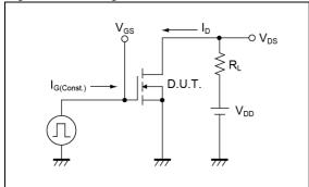
Fig.3-1 Avalanche Measurement Circuit
