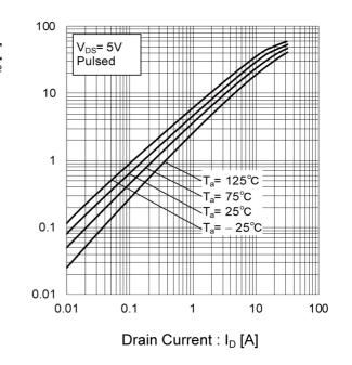
Fig.11 Drain Current Derating Curve
