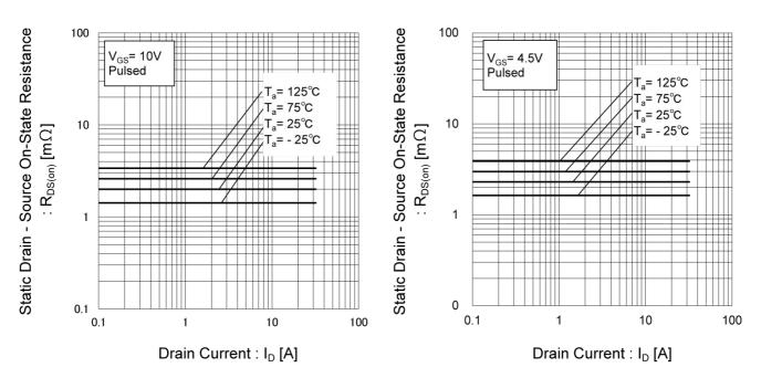
Fig.13 Static Drain - Source On - State Resistance vs. Junction Temperature Fig.14 Static Drain - Source On - State Resistance vs. Drain Current(I)
