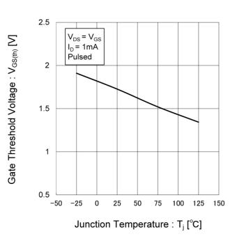
Fig.9 Gate Threshold Voltage vs. Junction Temperature
