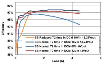
Figure 24. Boost Mode Efficiency
