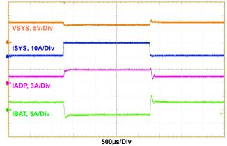
Figure 17. Buck Mode, Charge Current Loop to Adapter Current Loop Transition, V<sub>ADP</sub> = 20V, V<sub>BAT</sub> = 7V, MaxSystemVoltage = 8.384V, Adapter\_current\_limit = 3A, Charge\_current = 3A, System\_load = 0.5A to 10A
