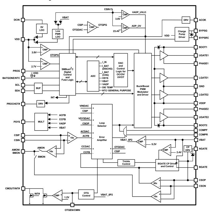
Figure 4. Block Diagram
