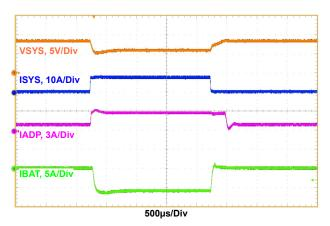
Figure 12. Boost Mode, Output Voltage Loop to Adapter Current Loop Transition, V<sub>ADP</sub> = 5V, V<sub>BAT</sub> = 7V, MaxSystemVoltage = 8.384V, Adapter\_current\_limit = 3A, Charge\_current = 0A, System\_load = 0.5A to 8A
