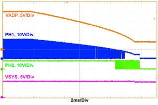
Figure 11. Adapter Voltage Ramp Down, Buck --> Buck\_Boost --> Boost Operation Mode Transition
