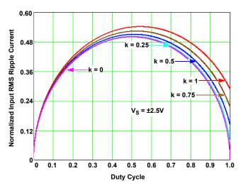
Figure 50. Normalized RMS Input Current at EFF = 1
