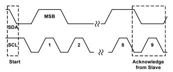
Figure 30. Acknowledge on the SMBus
