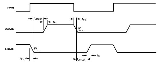
Figure 5. Gate Driver Timing Diagram
