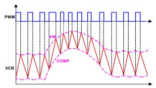
Figure 46. R3 Modulator Operation Principles in Dynamic Response
