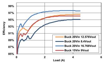
Figure 26. Buck Mode Efficiency
