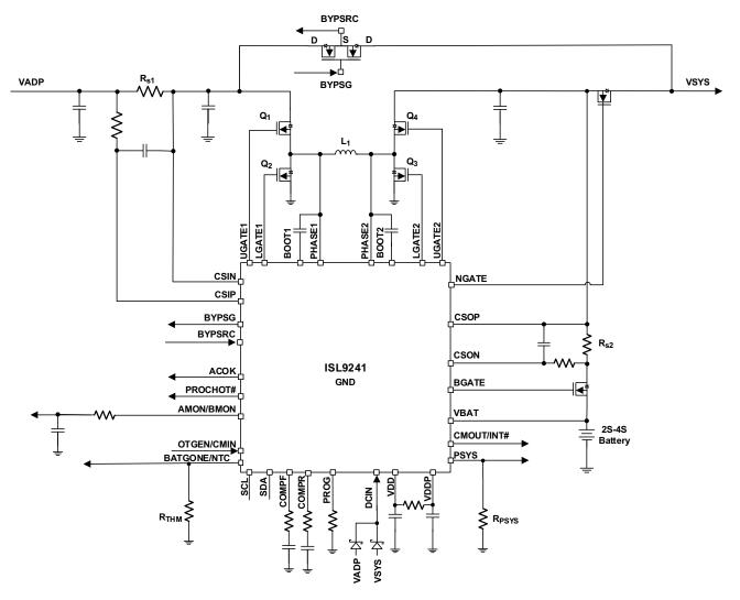
Figure 2. NVDC Plus HPBB Simplified Application Diagram
