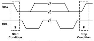
Figure 29. Start and Stop Waveforms
