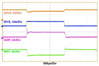
Figure 14. Buck\_Boost Mode, Output Voltage Loop to Adapter Current Loop Transition, V<sub>ADP</sub> = 9V, V<sub>BAT</sub> = 8.4V, MaxSystemVoltage = 8.8V, Adapter\_current\_limit = 3A, Charge\_current = 0A, System\_load = 0.5A to 8A
