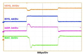
Figure 22. Bypass (HPBB) Mode, Reverse Turbo Boost Enabled. Output Voltage Loop to Adapter Current Limit Loop Transition. V<sub>ADP</sub> = 20V, V<sub>BAT</sub> = 8V, MaxSystemVoltage = 8.384V, Adapter\_current\_limit = 3A, Charge\_current = 0A, System\_load = 0.5A to 5A
