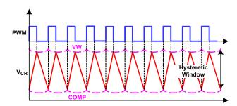
Figure 45. R3 Modulator Operation Principles in Steady State
