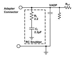
Figure 49. Adapter Input RC Snubber Circuit
