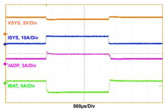
Figure 15. Buck\_Boost Mode, Charge Current Loop to Adapter Current Loop Transition, V<sub>ADP</sub> = 9V, V<sub>BAT</sub> = 8.4V, MaxSystemVoltage = 8.8V, Adapter\_current\_limit = 3A, Charge\_current = 1A, System\_load = 0.5A to 8A
