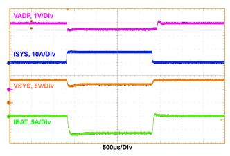
Figure 18. Boost Mode, Output Voltage Loop to Input Voltage Loop Transition, V<sub>ADP</sub> = 5V, V<sub>BAT</sub> = 8V, MaxSystemVoltage = 8.384V, Charge\_current = 0A, System\_load = 0.5A to 8A, Input\_voltage\_dac = 4.437V
