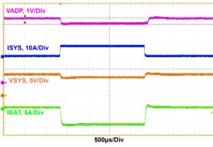
Figure 19. Boost Mode, Charge Current Loop to Input Voltage Loop Transition, V<sub>ADP</sub> = 5V, V<sub>BAT</sub> = 8V, MaxSystemVoltage = 8.384V, Charge\_current = 0.5A, System\_load = 0.5A to 8A, Input\_voltage\_dac = 4.437V
