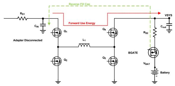
Figure 35. Supplemental Mode Energy Flow
