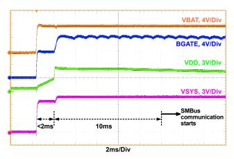
Figure 6. Start Up Time with Battery for Communication
