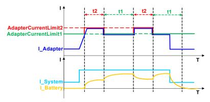
Figure 43. Two-Level Adapter Current Limit
