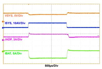
Figure 13. Boost Mode, Charge Current Loop to Adapter Current Loop Transition, V<sub>ADP</sub> = 5V, V<sub>BAT</sub> = 7V, MaxSystemVoltage = 8.384V, Adapter\_current\_limit = 3A, Charge\_current = 0.5A, System\_load = 0.5A to 8A
