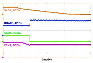
Figure 9. Adapter Removal. V<sub>ADP</sub> = 5V, MaxSystemVoltage = 8.384V, V<sub>BAT</sub> = 7V, Charge Current Limit = 0A, System load = 20mA
