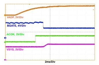
Figure 8. Start Up with Adapter and Battery. V<sub>ADP</sub> = 5V, MaxSystemVoltage = 8.384V, V<sub>BAT</sub> = 7V, Charge Current Limit = 0A
