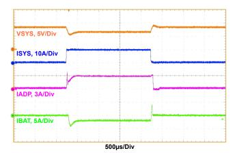
Figure 16. Buck Mode, Output Voltage Loop to Adapter Current Loop Transition, V<sub>ADP</sub> = 20V, V<sub>BAT</sub> = 7V, MaxSystemVoltage = 8.384V, Adapter\_current\_limit = 3A, Charge\_current = 0A, System\_load = 0.5A to 10A
