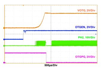
Figure 20. OTG Mode Enable Using OTGEN Pin.
