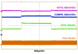
Figure 21. OTG Mode Transient. V<sub>BAT</sub> = 8V, V<sub>OTG</sub> = 5V, OTG Current = 3.2A, Load = 0.5A to 3A
