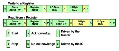
Figure 31. SMBus Read and Write Protocol
