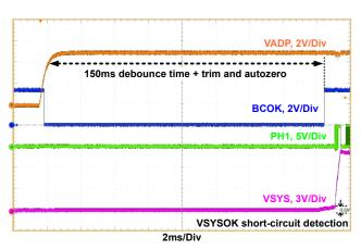
Figure 7. Start Up with 5V Adapter and ACOK Timing
