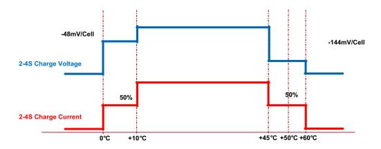
Figure 32. JEITA Profile for 2-4 Cell Battery
