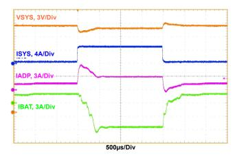
Figure 23. Bypass (HPBB) Mode, Reverse Turbo Boost Enabled. Charge Current Loop to Adapter Current Limit Loop Transition. V<sub>ADP</sub> = 20V, V<sub>BAT</sub> = 8V, MaxSystemVoltage = 8.384V, Adapter\_current\_limit = 3A, Charge\_current = 2A, System\_load = 0.5A to 5A
