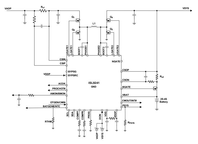
Figure 3. NVDC Only Simplified Application Diagram
