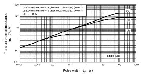
Fig. 8.13 r<sub>th</sub> - t<sub>w</sub> (Guaranteed Maximum)
