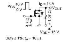
Fig. 6.2.1 Switching Time Test Circuit
