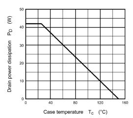
Fig. 8.12 P<sub>D</sub> - T<sub>c</sub> (Guaranteed Maximum)
