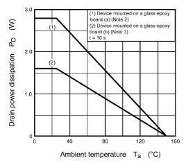
Fig. 8.11 P<sub>D</sub> - T<sub>a</sub> (Guaranteed Maximum)
