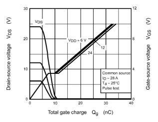
Fig. 8.10 Dynamic Input/Output Characteristics
