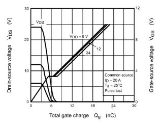
Fig. 8.10 Dynamic Input/Output Characteristics
