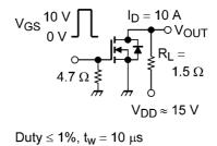
Fig. 6.2.1 Switching Time Test Circuit
