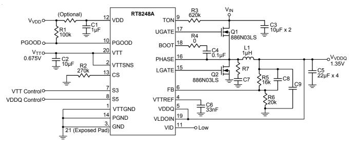
Figure 2. Typical Application Circuit with Pure MLCC Solution
