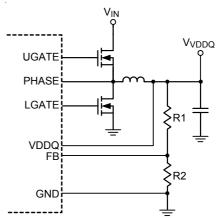
Figure 6. Setting VDDQ with a Resistive Voltage Divider
