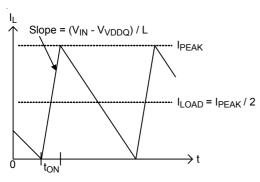
Figure 3. Boundary Condition of CCM/DCM
