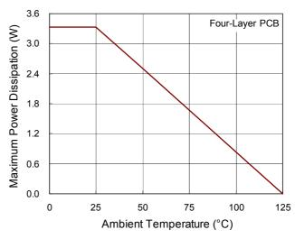
Figure 7. Derating Curve of Maximum Power Dissipation
