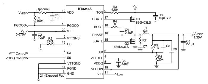
Figure 1. Typical Application Circuit with POSCAP Solution
