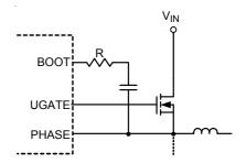
Figure 5. Increasing the UGATE Rise Time
